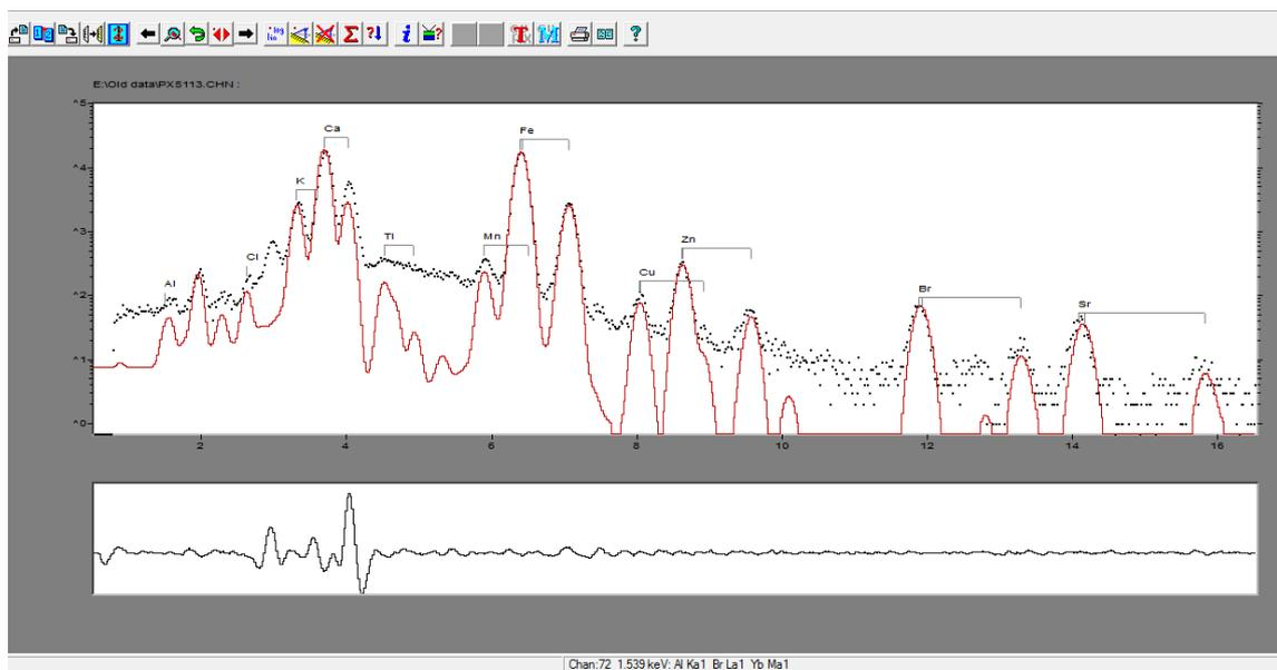
Figure 2: Analyzed data spectrum of a powder milk sample
