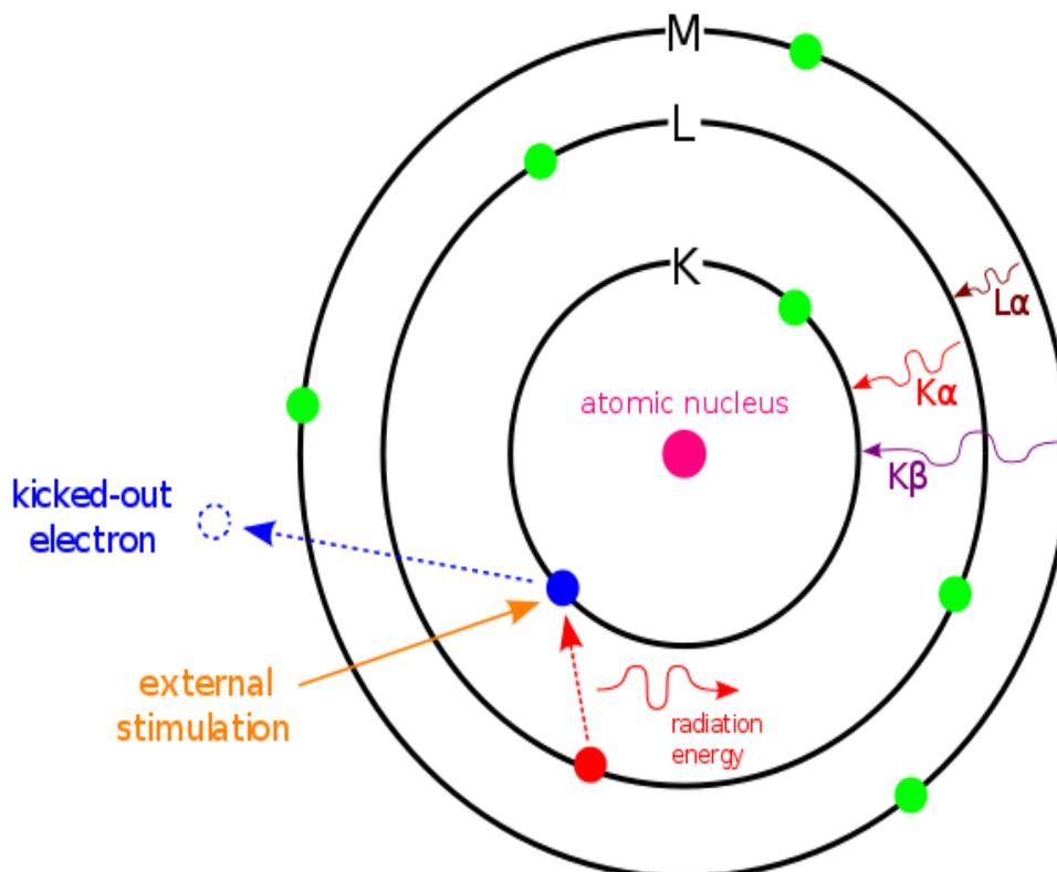
Figure 1: Characteristic X-ray emission by incident proton beam
