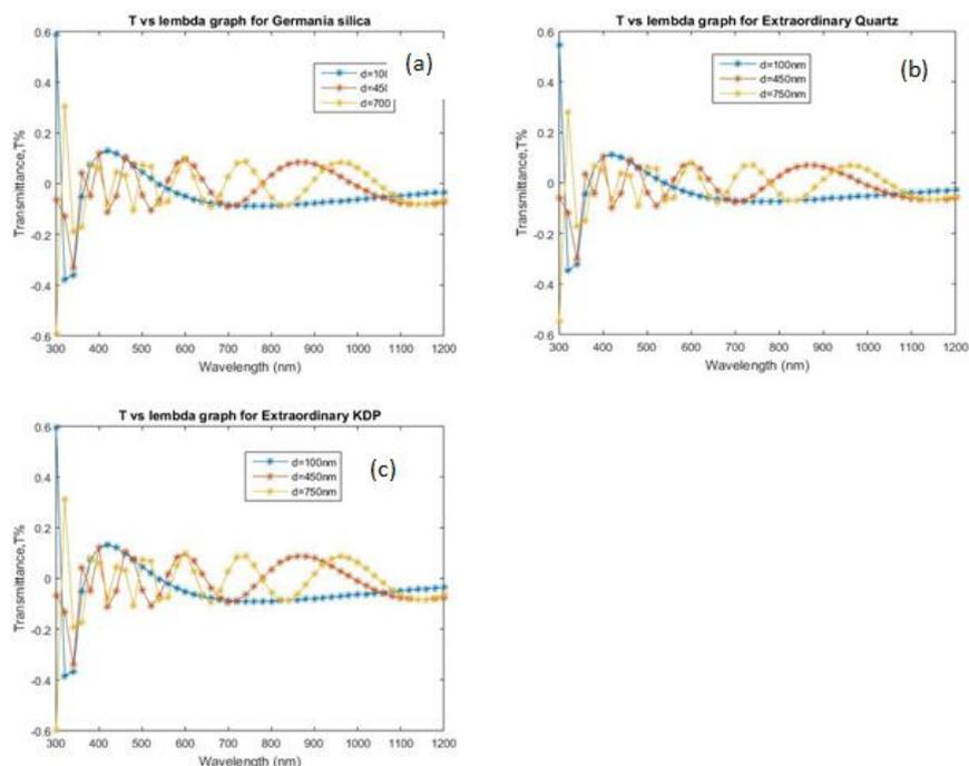
**Figure 6 :** Transmission spectrum( with interference effect ) of ZnO thin film for different thicknesses deposited on (a) Germania Silica,(b) extraordinary quartz, and (c)extraordinary KDP.
