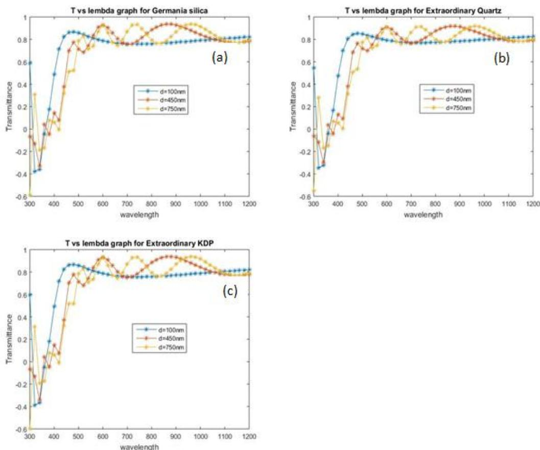
**Figure 4:** Transmission spectrum of ZnO thin film for different thicknesses deposited on (a) Germania Silica, (b) extraordinary quartz, and (c) extraordinary KDP.
