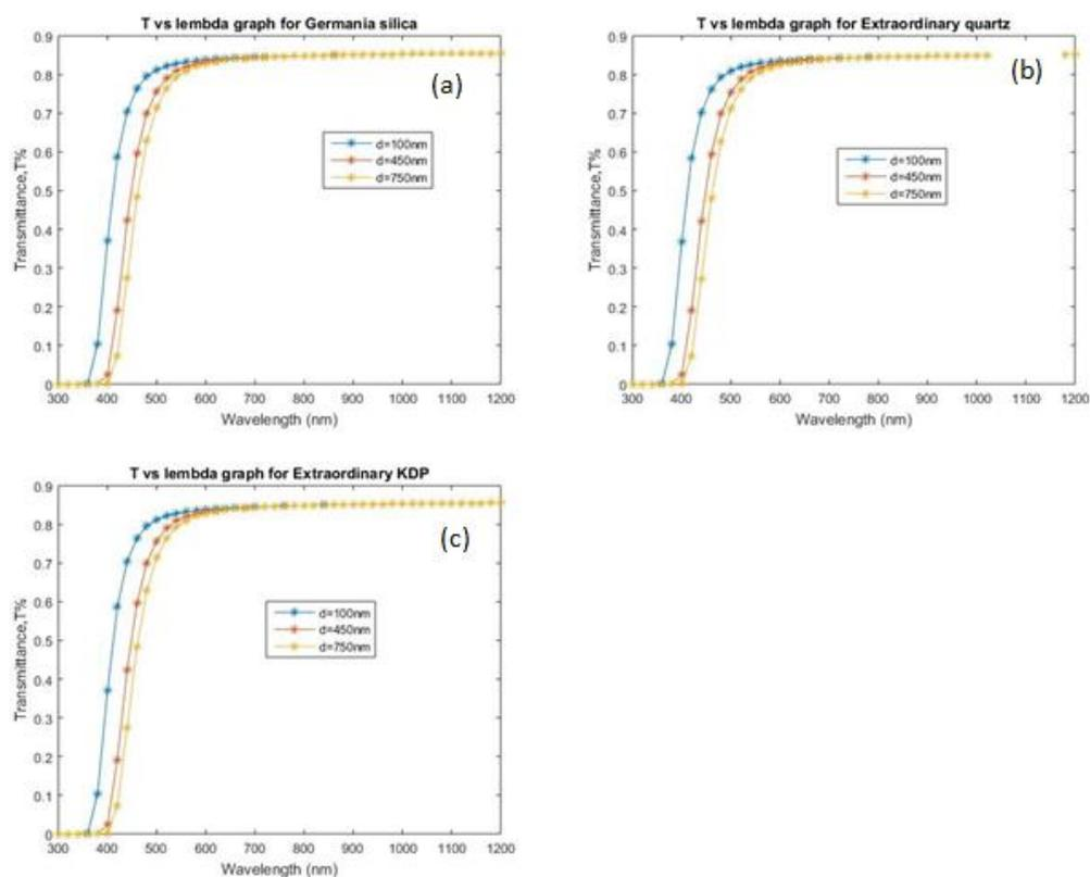
**Figure 5:** Transmission spectrum without interference effect of ZnO thin film for different thicknesses deposited on (a) Germania Silica, (b) extraordinary quartz, and (c) extraordinary KDP.
