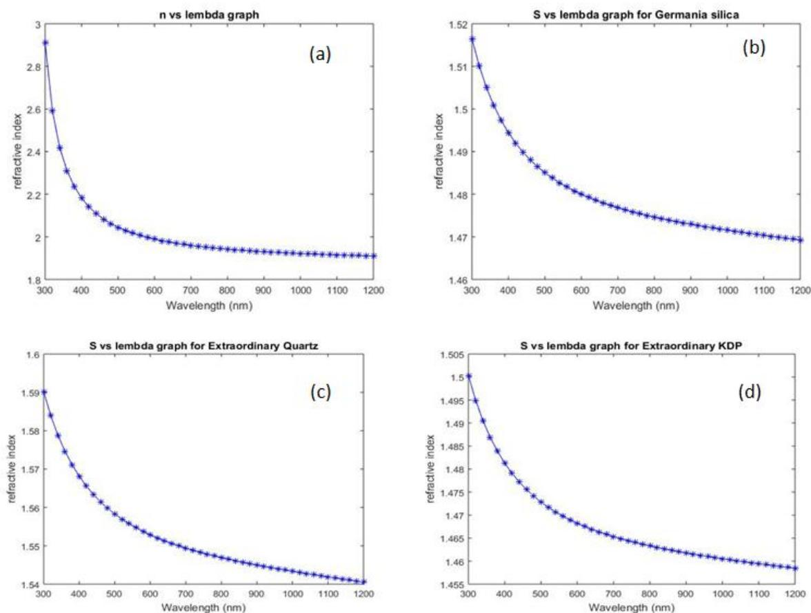
**Figure2:** Variation of refractive index as a function of wavelength for (a)ZnO, (b)Ge-Si, (c)Extraordinary Quartz, (d)Extraordinary KDP.
