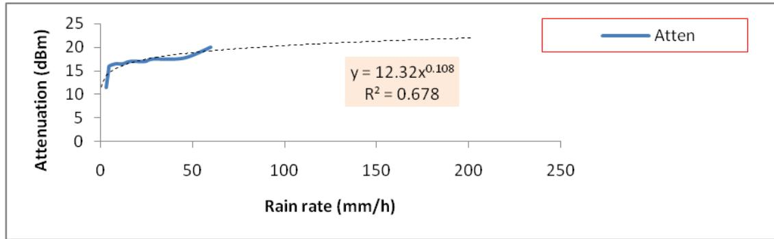
**Figure 5:** Model - Rain attenuation as a function of rain rate, Sep 2014.
