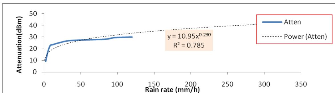
Figure1: Model – Rain attenuation as function of rain rate, Apr 2014.
