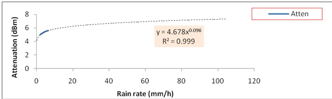
Figure 6: Model -Rain attenuationas function of rain rate, Oct 2014.
