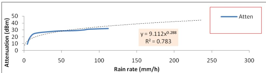
Figure 7: Model – Rain attenuationas function of rain rate for the year 2014.
