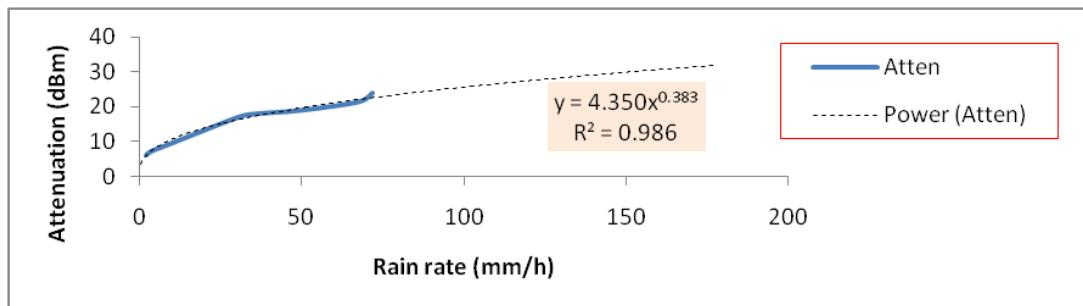
**Figure 2:** Model – Rain attenuation as a function of rain rate for May 2014.
