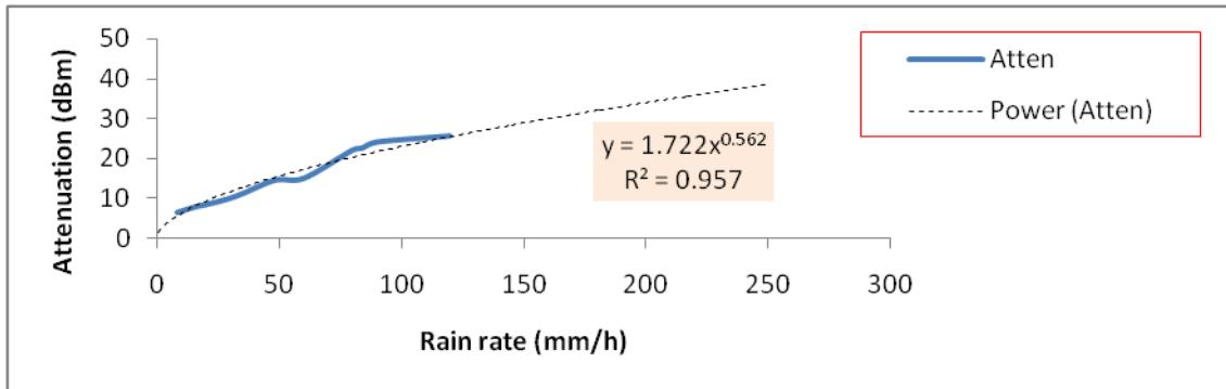
**Figure 4:** Model of rain attenuation as a function of rain rate Jul 2014.
