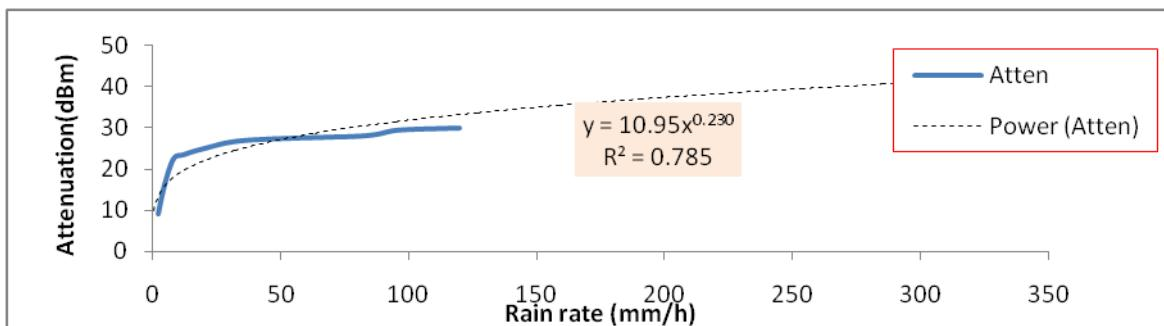
Figure1: Model – Rain attenuation as function of rain rate, Apr 2014.
