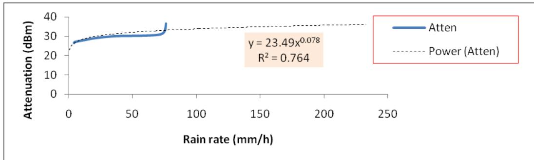
**Figure 3:** Model – Rain attenuation as a function of rain rate Jun 2014.
