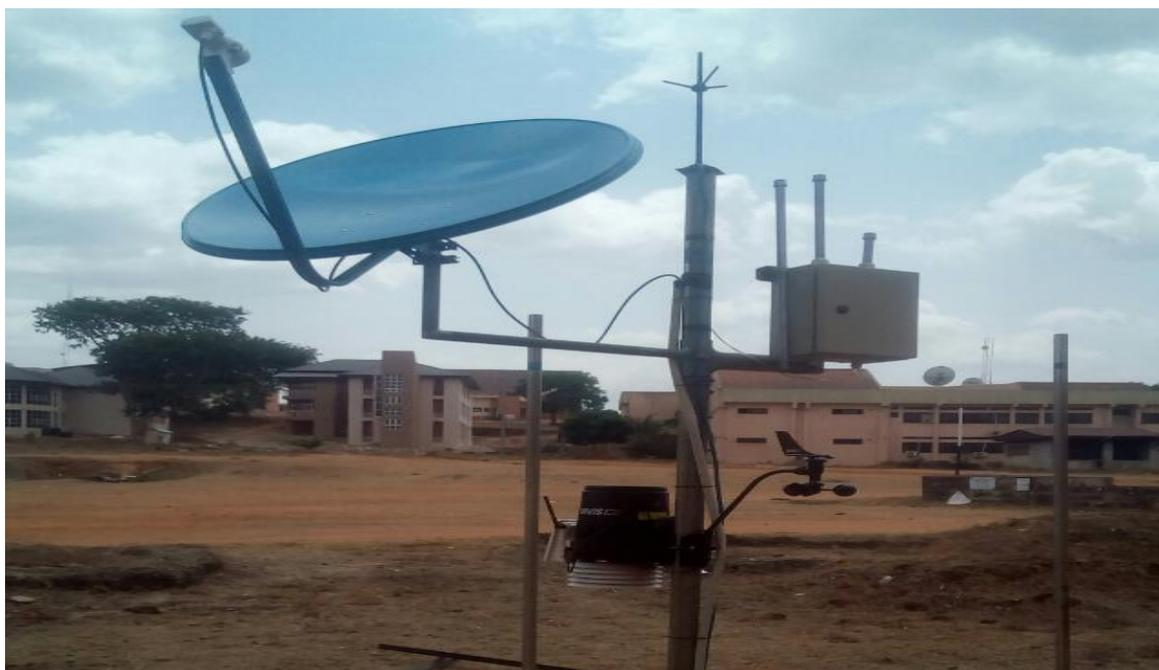
**Figure 1.** Automated Weather Station.
