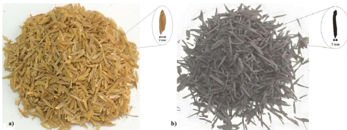
Figure 4: Samples of Rice Husk (RH) before (a) and after (b) Pyrolysis
