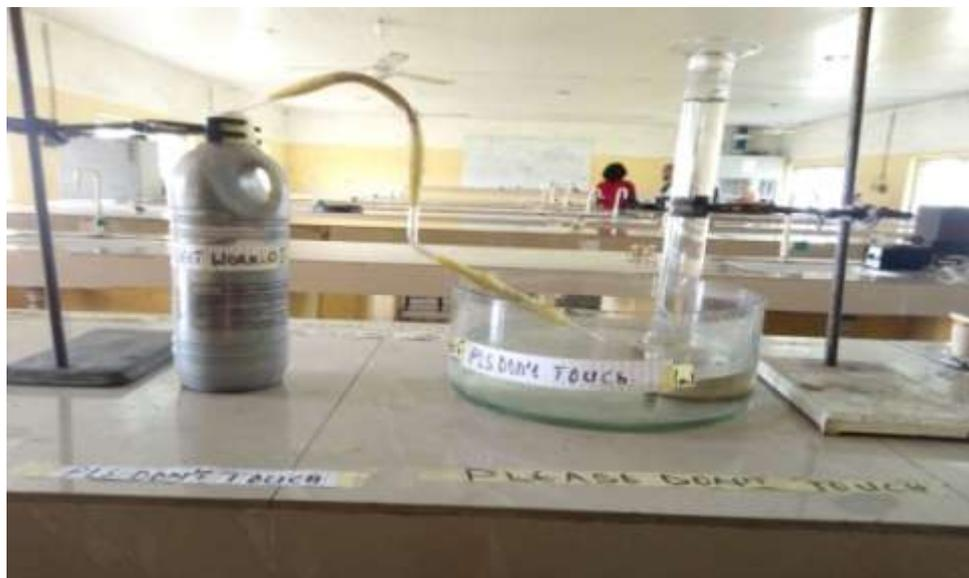
**Figure 2:** Experimental Set-Up For Biogas Production
