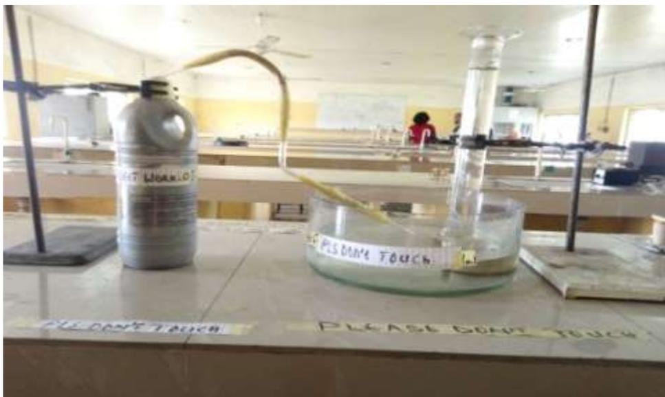
**Figure 2:** Experimental Set-Up For Biogas Production
