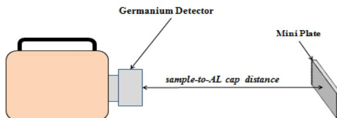
Fig. 2: A schematic diagram for the configuration of targets during measurement.
