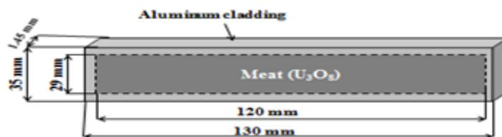
Fig. 1: shape and example for dimensions of the assayed targets
