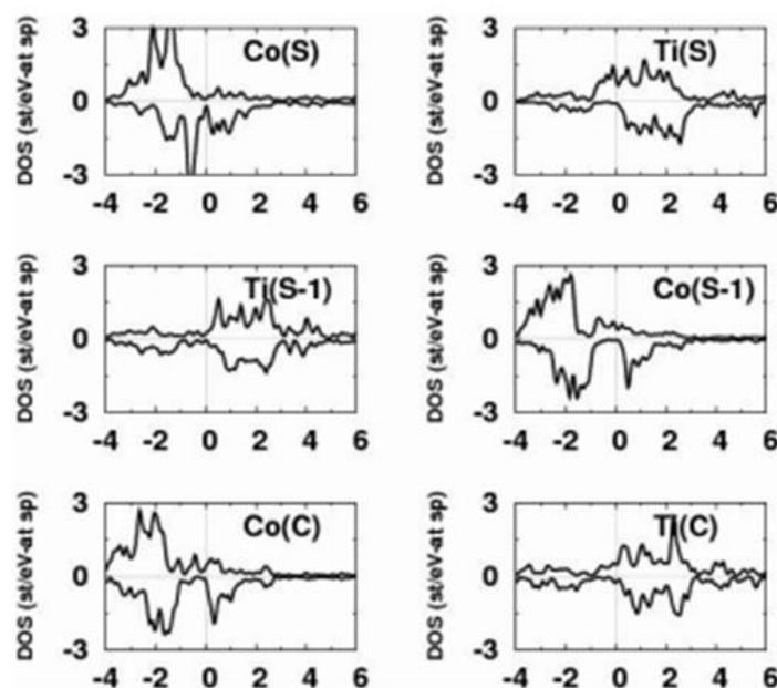
**Fig. 1** Atom-projected spin-polarized density of states (DOS) for the chosen atoms of the Co- (left-panels) and Ti-terminated (right-panels) CoTi(001) surface. The spin-down DOS values are multiplied by a negative number, and the Fermi levels are set to zero.
