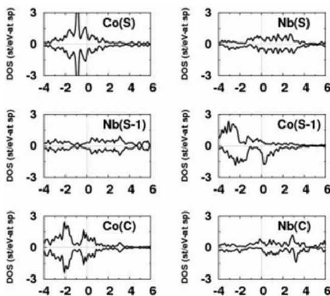
**Fig. 3** Atom-projected spin-polarized density of states (DOS) for the chosen atoms of the Co- (left-panels) and Nb-terminated (rightpanels) CoNb(001) surface. The spin-down DOS values are multiplied by a negative number, and the Fermi levels are set to zero.
