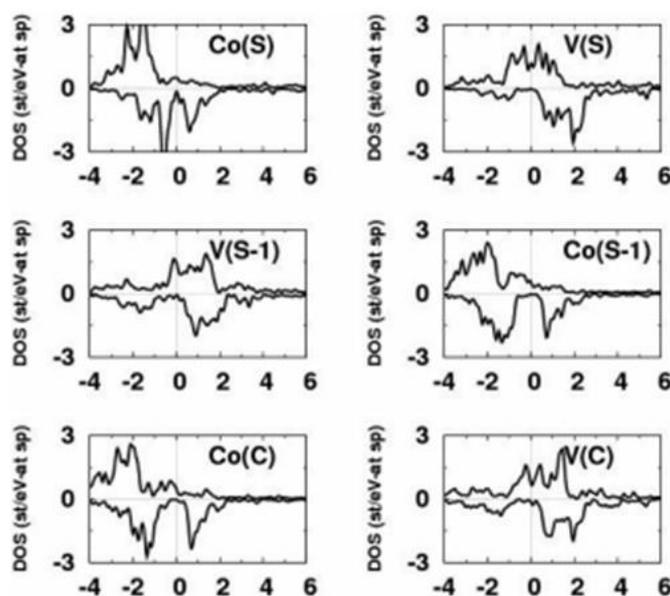
**Fig. 2** Atom-projected spin-polarized density of states (DOS) for the chosen atoms of the Co- (left-panels) and V-terminated (right-panels) CoV(001) surface. The spin-down DOS values are multiplied by a negative number, and the Fermi levels are set to zero.
