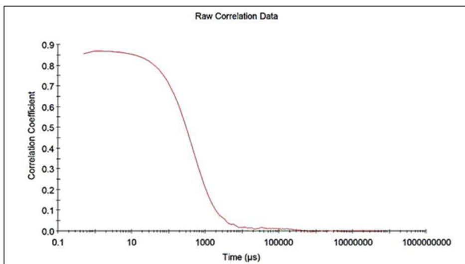
Figure 7 Correlogram for the cumulants for the ZnO nanoparticles
