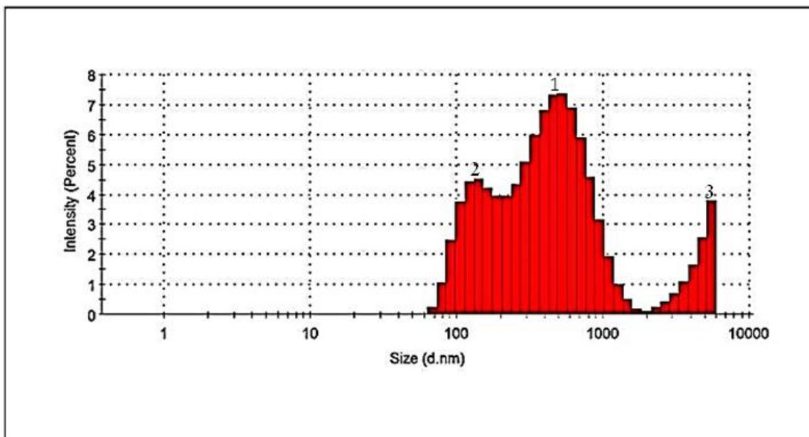
**Figure 3** Size distributions of ZnO nanoparticles by intensity
