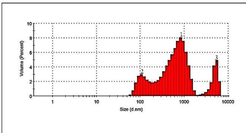
**Figure 2** ZnO nanoparticles size distributions by volume
