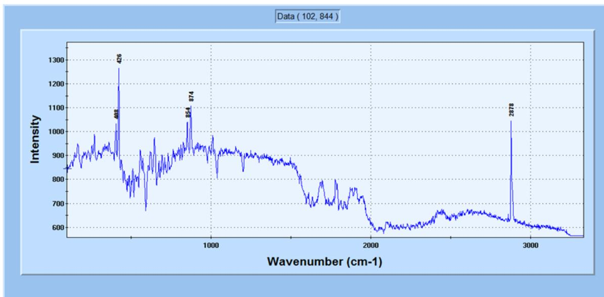
**Figure 1** Raman spectrum of the synthesized ZnO nanoparticles
