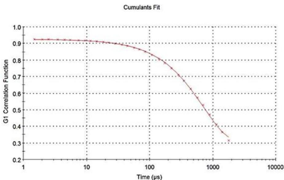
Figure 8: Cumulants fit for the ZnO nanoparticles
