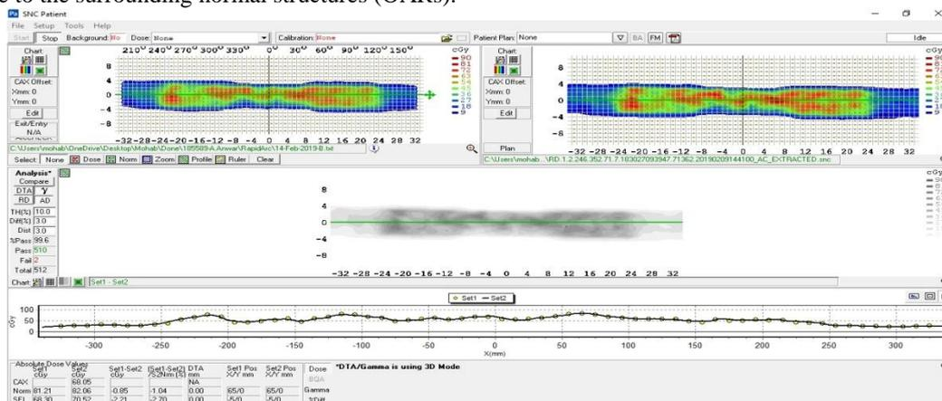
**Fig 1:** 2D dose analysis generated by SNC patient software shows measured ArcCHECK dose points
