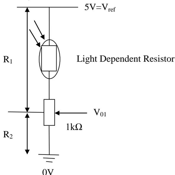
**Figure 3.1.1:** Light Intensity Circuit
