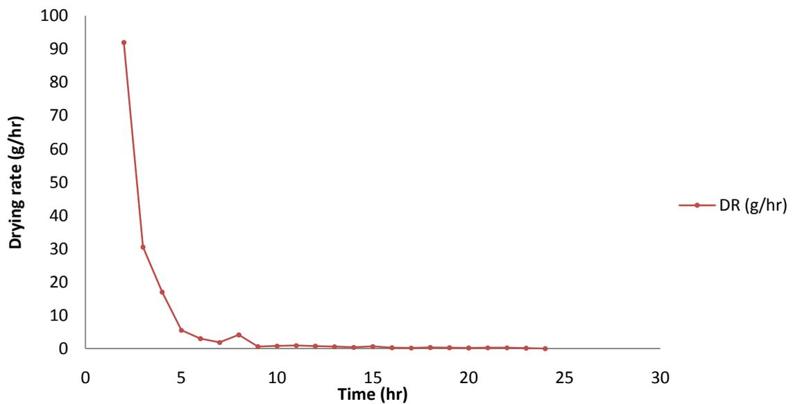
Figure 4.3: Drying rate with time of sliced Yam in the solar concentrator dryer
