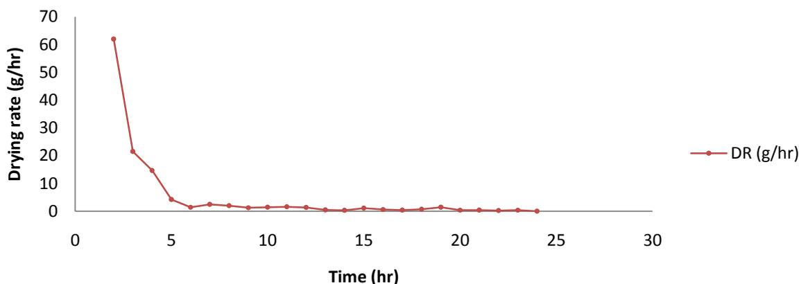
**Figure 4.5:** Drying rate with time of sliced Yam in the open sun
