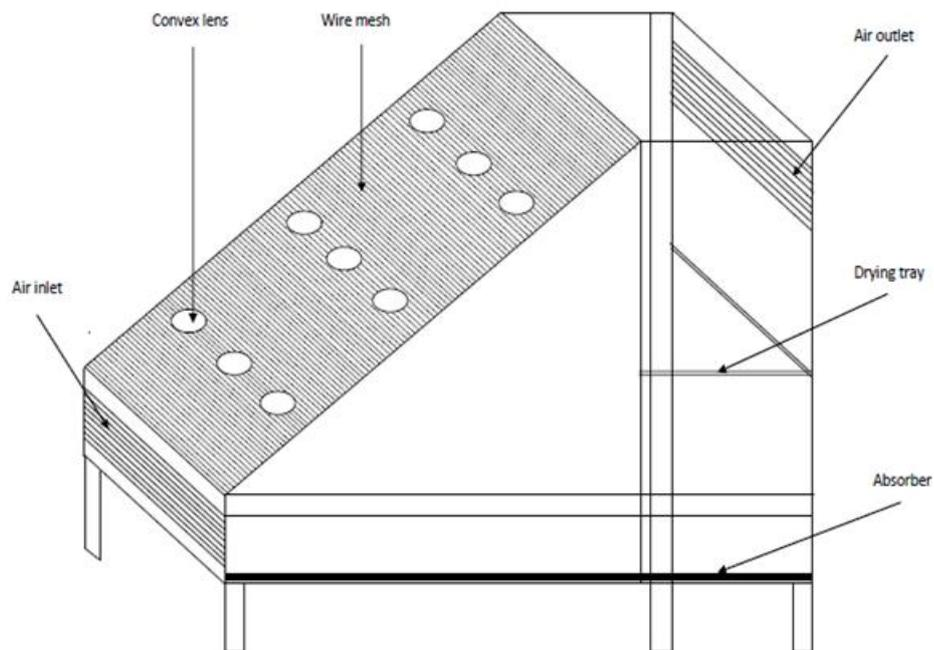
**Figure 3:** Schematic diagram of the solar concentrator dryer.
