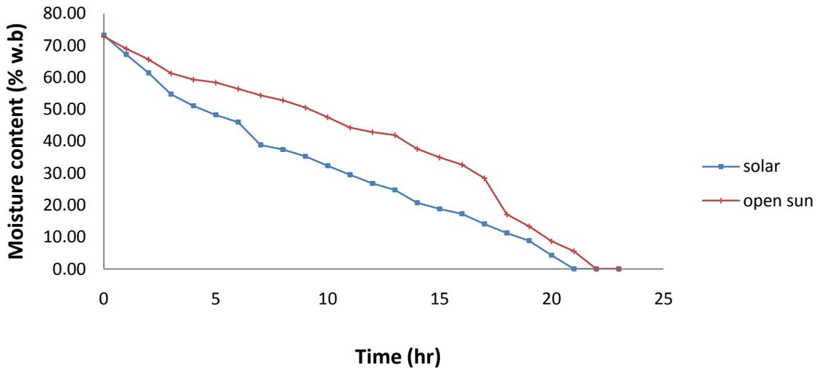
Figure 4.2: Variation of moisture content of sliced Yam in the solar concentrator dryer and open sun
