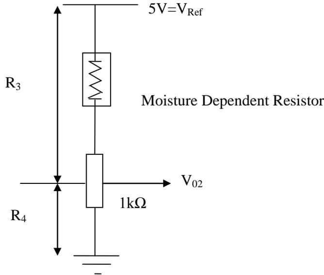
Figure 3.1.2: Moisture Content Measurement Circuit
