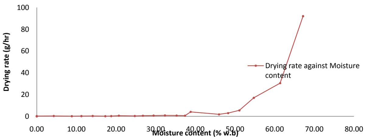
Figure 4.4: Drying rate with moisture content of sliced Yam in the solar concentrator dryer
