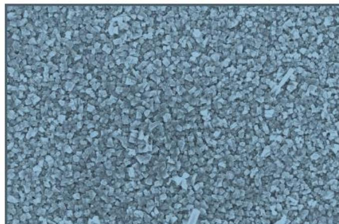
Figure 2: Scanning electron microscopic image of synthesized ZnOnano structures
