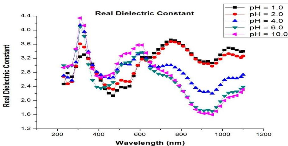
Figure 9: The plot of the real dielectric constant against wavelength for pH variation of PANI CMC samples
