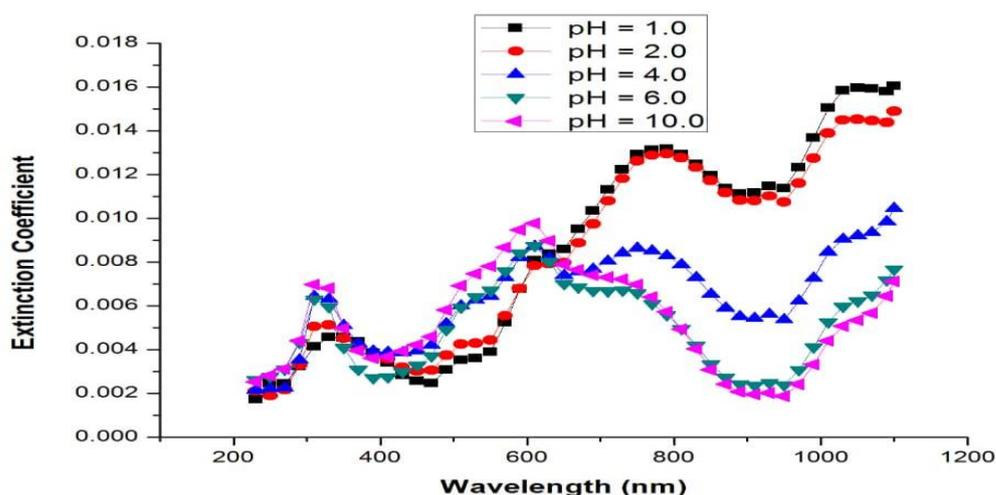
Figure 8: Plot of extinction coefficient values versus wavelength for different pH samples variation.
