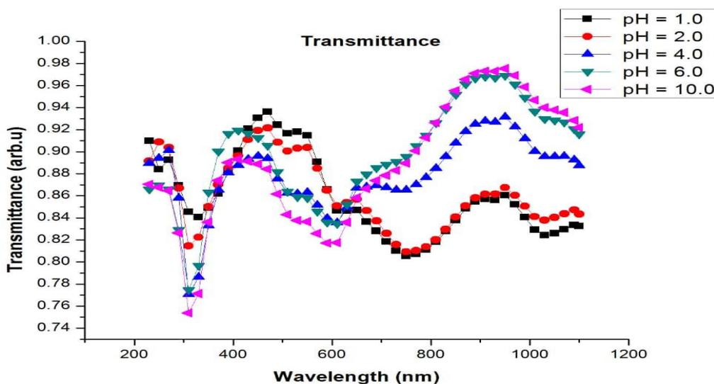
Figure 3: Transmission spectra for PANI CMC samples at different pH Variation.
