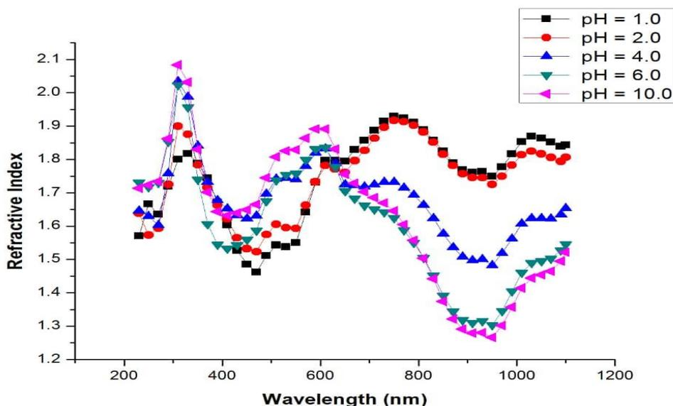
**Figure 6: Plot of refractive index versus wavelength for PANI CMC samples at different pH variations**
