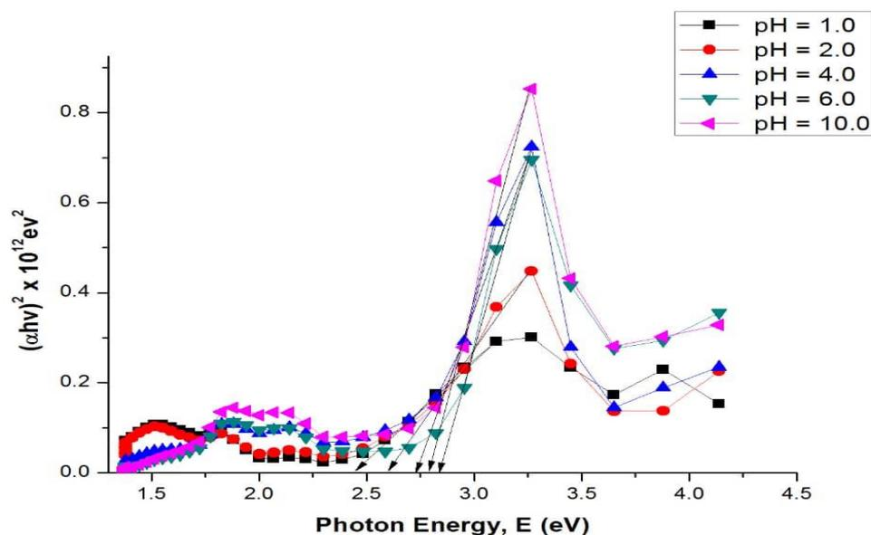
Figure 2: Plot of  $(\alpha h\nu)^2$  versus photon energy for pH variations of PANI CMC samples
