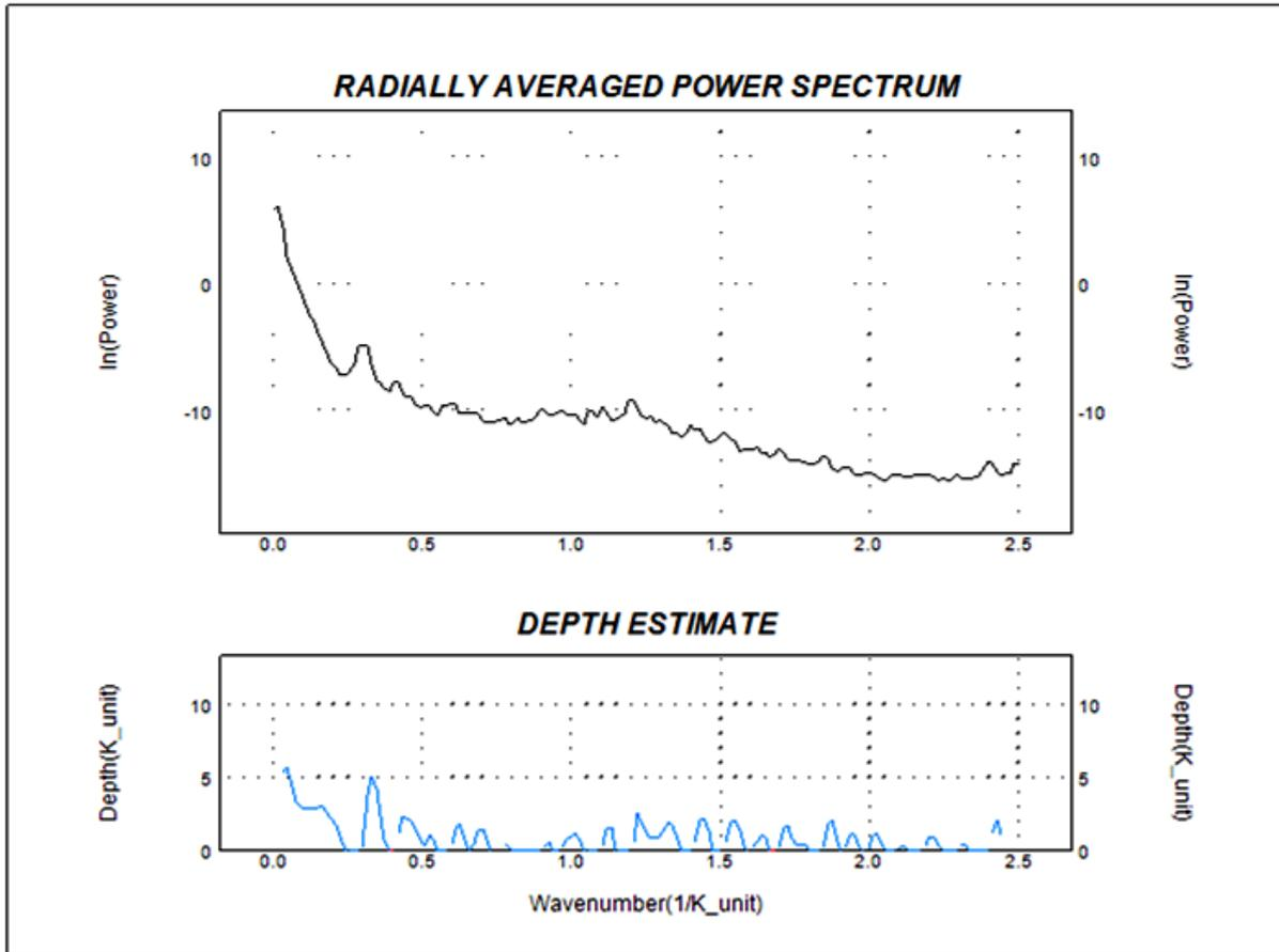
Fig. 7: Radial average power spectrum for the gravity data
