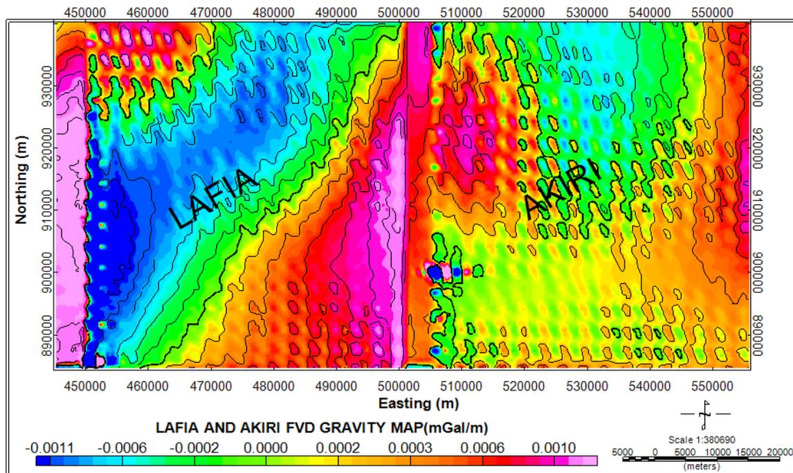
Fig. 4: Aerogravity First Vertical Derivative (FVD)
