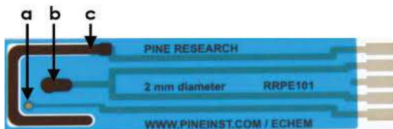
Fig. 8. Pine screen printed electrode. (a)-Counter Electrode,(b)-Working Electrode,(c)-Reference Electrode
