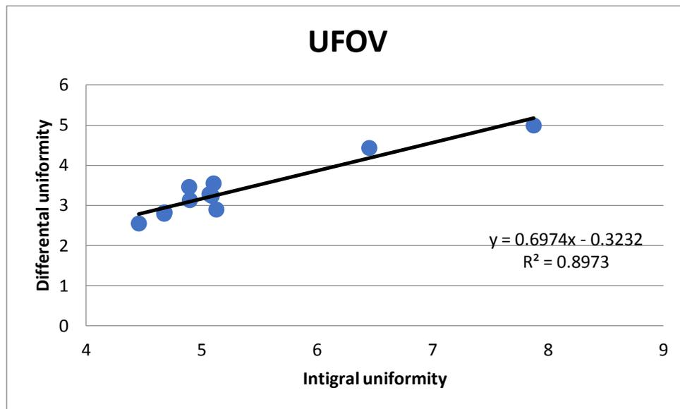
Figure 1. scatter plot show a direct linear relationship of DU of UFOV with IU
