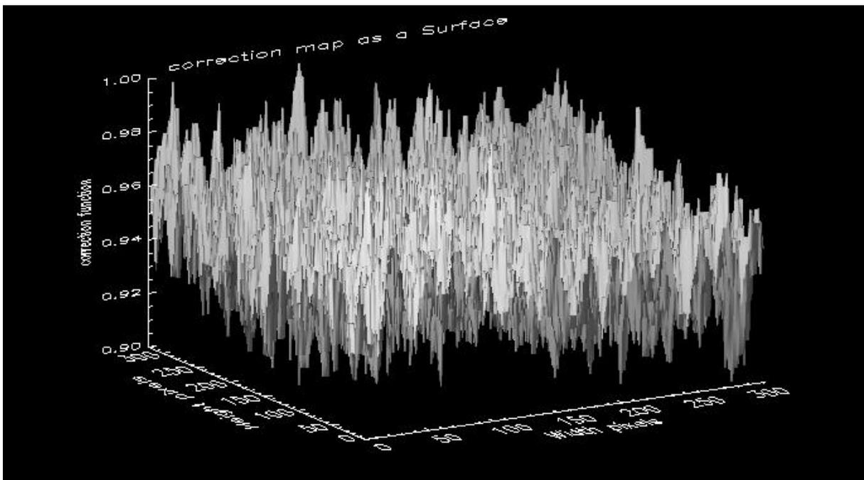
Figure 4. shade-surface of the correction matrix that used to overcome the problem of uniformity if the value of uniformity exceeds the limits.
