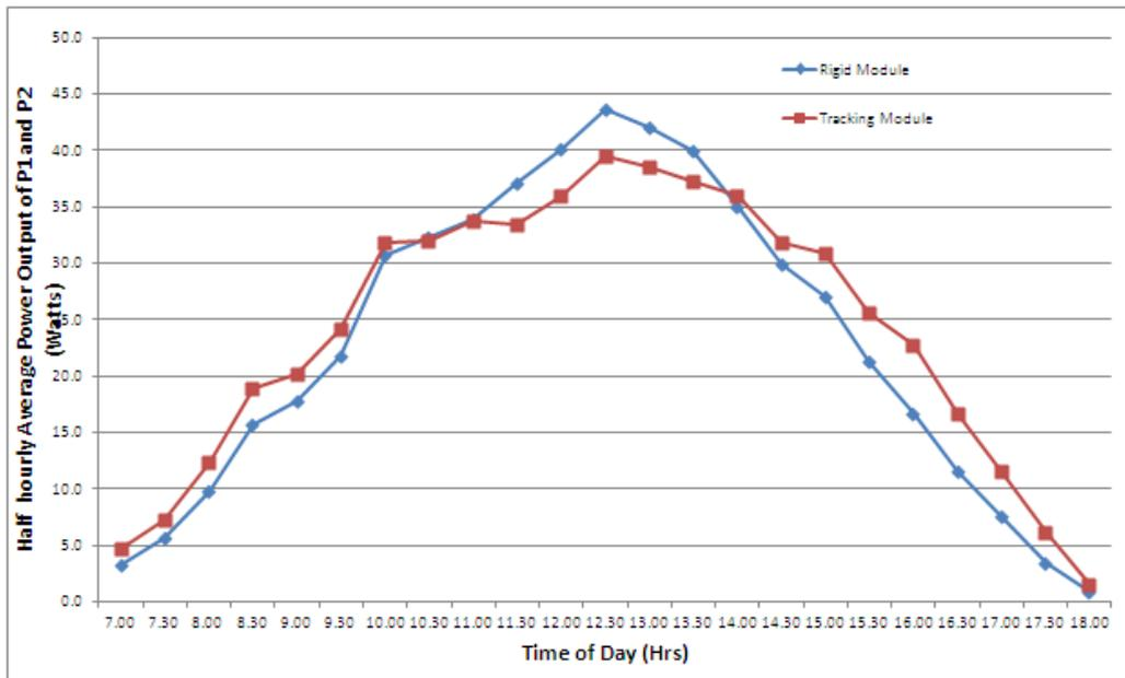
Fig. 9 Half Hourly Average Power-Output of Modules (Watt) against Time of Day (hrs)
