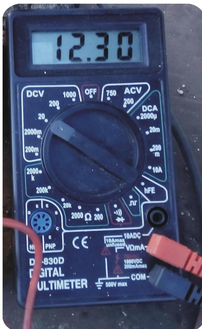
**Fig. 7 Digital Multi-meter in Voltage Measuring Mode**
