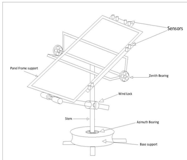
Fig. 3 Diagram of the Tracking Mount
