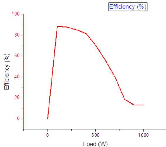
Fig. 2 b: Variation of Efficiency with Loads (0 W – 1000 W)
