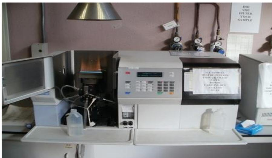
Fig. 1: Atomic Absorption Spectrophotometer Set-Up
