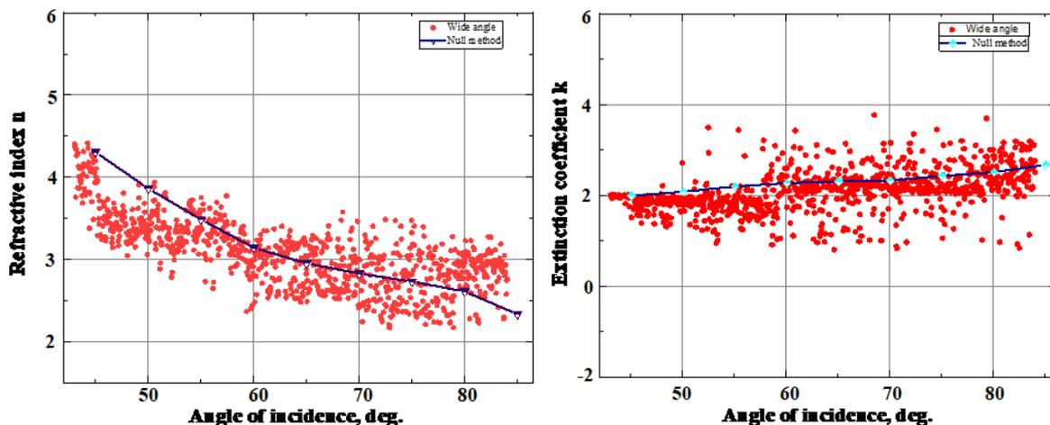
Fig. 3. The optical constants  $n, k$  at different angle of incidence for Cd sample measured by wide angle experiment and null ellipsometric method.
