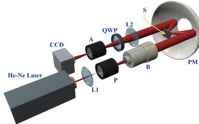
Fig. 1 The optical arrangement of the developed wide angle of incidence ellipsometric setup which consists of: He-Ne Laser at 633 nm; L1, L2: two convex lenses; P, A: Glan-Thompson polarizer and analyzer; B: beam expander; PM: parabolic mirror; S: sample; QWP: quarter wave plate; CCD: CMOS camera.
