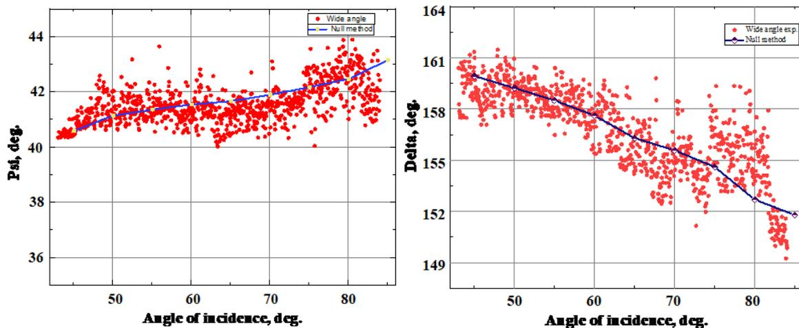
Fig. 2. The ellipsometric parameters  $\Psi, \Delta$  at different angles of incidence for cadmium sample by wide angle experiment and null ellipsometric method.
