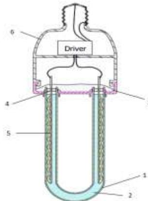
**Figure 1:** Structure of LED heat dissipation by self-convection
