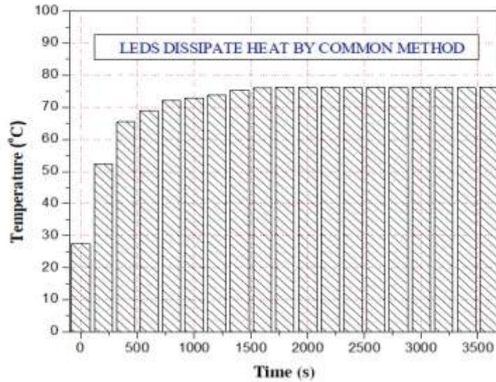
**Figure 3:** Temperatures of LED chip according to its operating time when using common heat dissipation method
