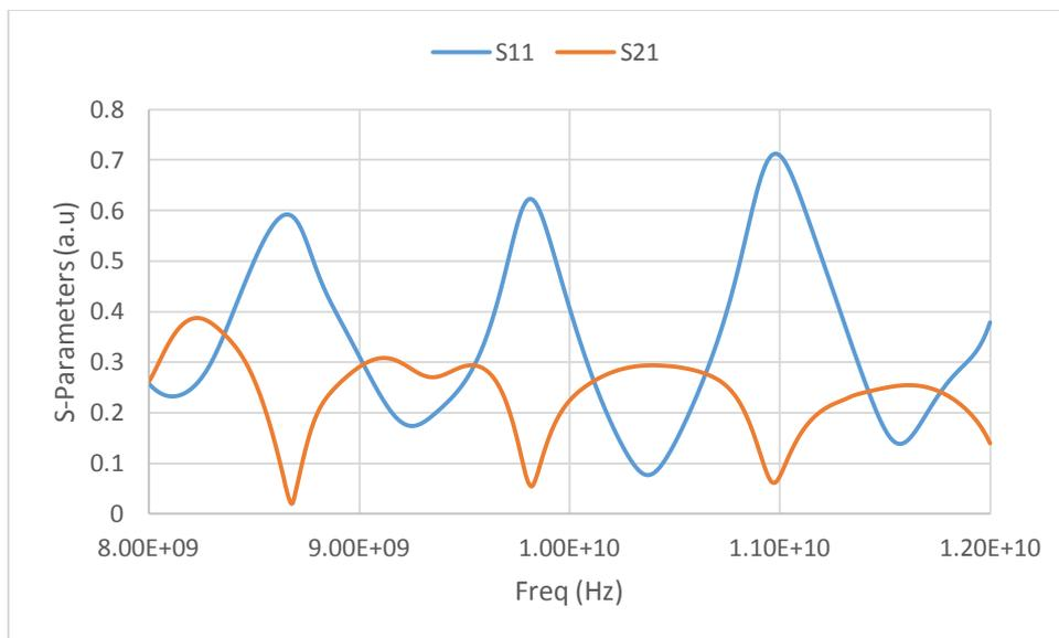
Figure 6: S-Parameter of Duroid at 4.5 Permittivity
