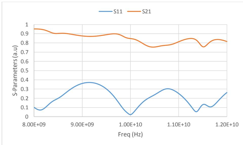
**Figure 2: S-Parameter of Duroid at 2.5 Permittivity**
