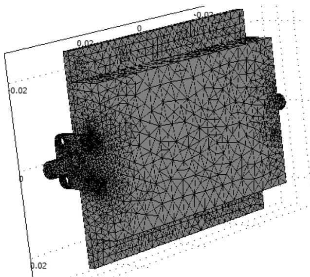
**Figure 1: High Mesh Density of an Overlay Microstrip Antenna**
