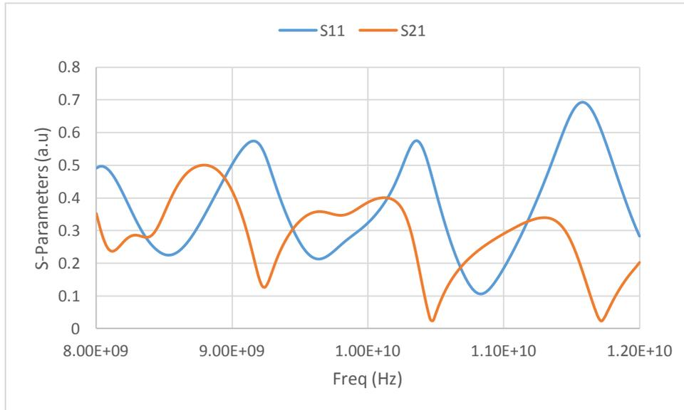
Figure 5: S-Parameter of Duroid at 4.0 Permittivity
