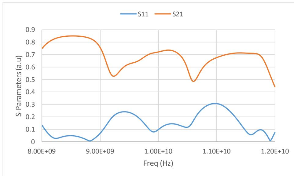
**Figure 3: S-Parameter of Duroid at 3.0 Permittivity**
