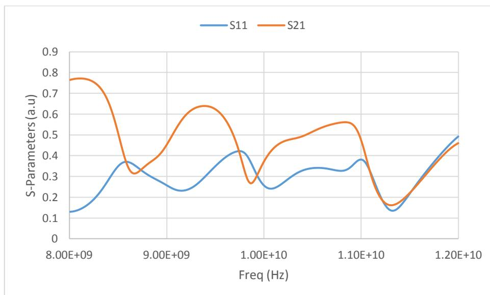
**Figure 4: S-parameter of Duroid at 3.5 Permittivity**
