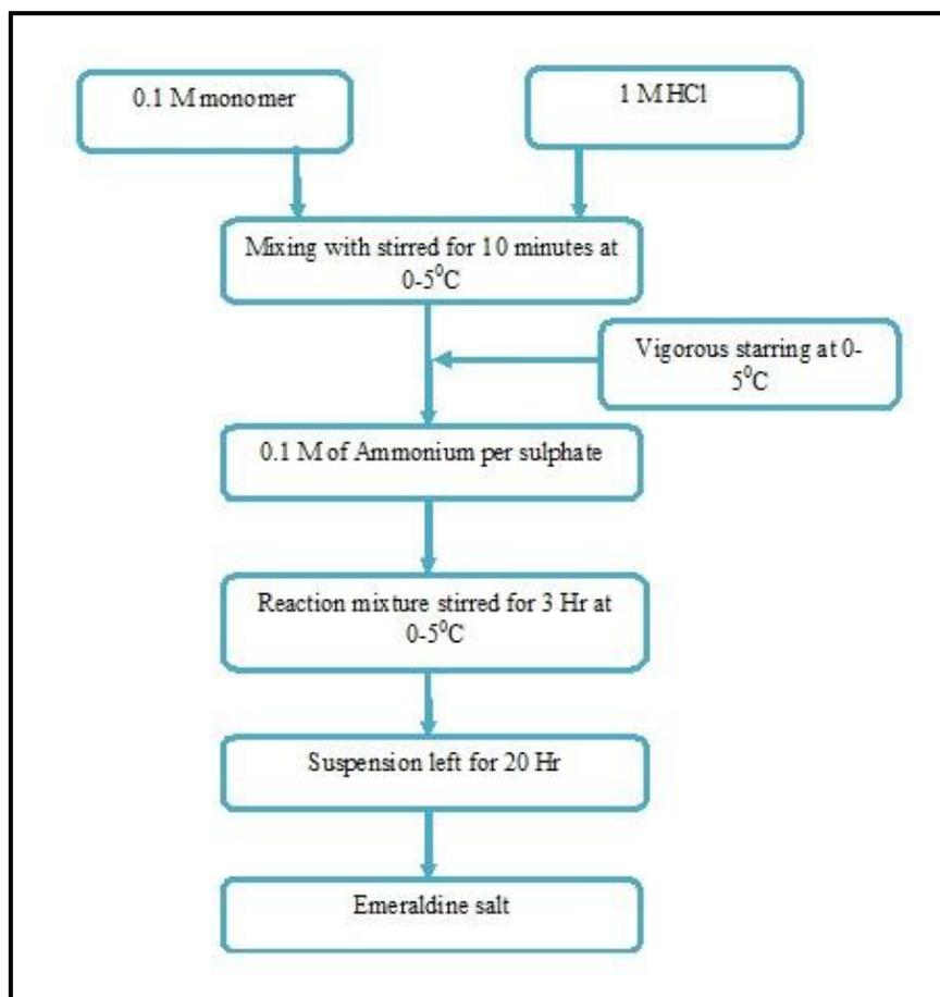
**Fig. 1: Flow chart for the synthesis of polymer by *in situ* polymerization method.**
