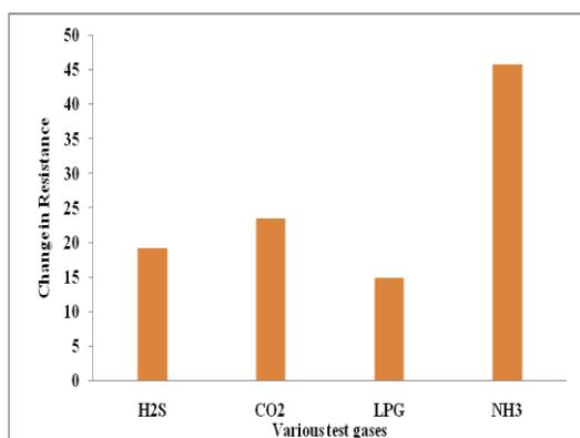
Figure 7: Variation of sensitivity for various gases test gases
