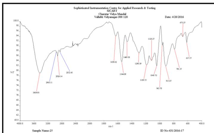
Fig 2: FTIR spectra pure PPy
