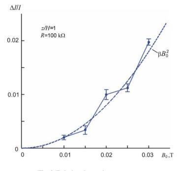
Fig. 3. Relative change in current as a function of magnetic field induction.
