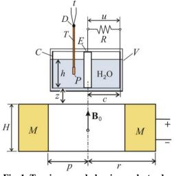
Fig. 1. Two immersed aluminum electrodes in magnetic field of electromagnet *M*.
