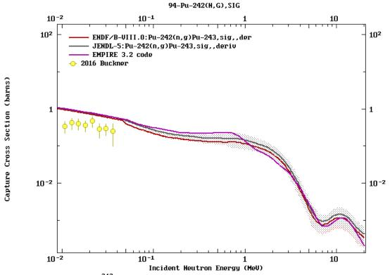
Figure 5: The spectrum of  $^{242}Pu(n, \gamma)$  cross section (barns) as a function of neutron incident energy (MeV)
