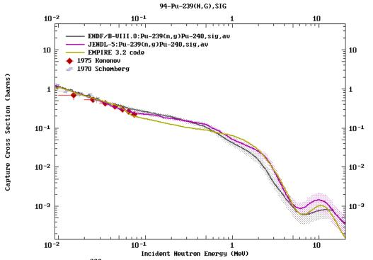
Figure 2: The spectrum of  $^{239}Pu(n, \gamma)$  cross section (barns) as a function of neutron incident energy (MeV)
