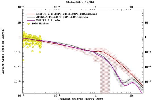
Figure 4: The spectrum of  $^{241}Pu(n, \gamma)$  cross section (barns) as a function of neutron incident energy (MeV)
