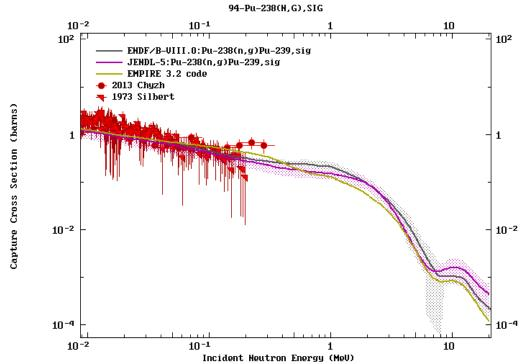
Figure 1: The spectrum of  ${}^{238}Pu(n, \gamma)$  cross section (barns) as a function of neutron incident energy (MeV)
