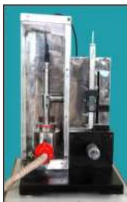
Fig. 3: Sample Holder for Ultrasonic Attenuation and Velocity Measurement in Liquids
