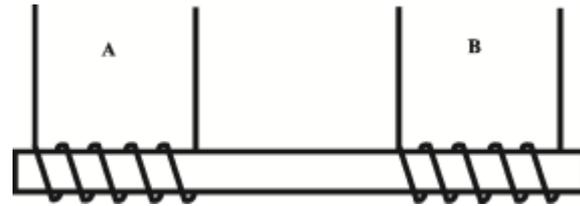
Fig. 1. The simple form of the magnetic fluxgate sensor
