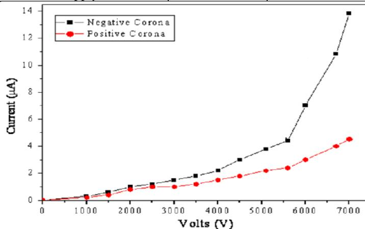
Fig. 2 V-I Characteristic of corona ionization
