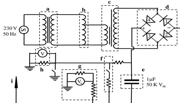
Fig.1. Schematic layout of the power supply a) isolation transformer b) autotransformer c) neon transformer d) bridge rectifier e) high voltage capacitor f) capacitor discharge system g) high voltage measurement system h) current measurement system i) discharge electrode
