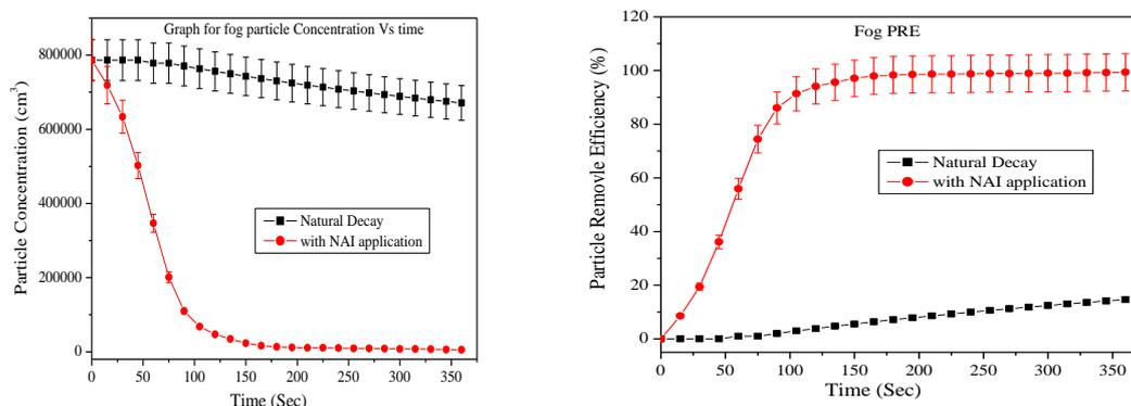
Fig. 3 Particle concentration & PRE verses time with natural decay and negative discharge (NAI) application for fog.
