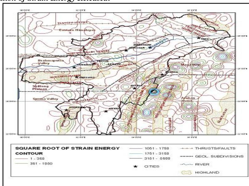
**Figure 10: Iso-strain energy (ergs) x  $10^7$  release map of the study region with grid  $\{(1)^0 \times (1)^0\}$**
