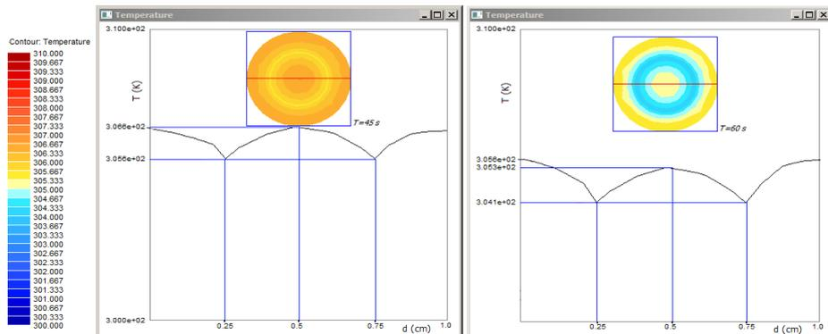
Fig. 8: Images of temperature for  $t=45$  s and  $t=60$  s across the specimen,  $d$  (normalized diameter).
