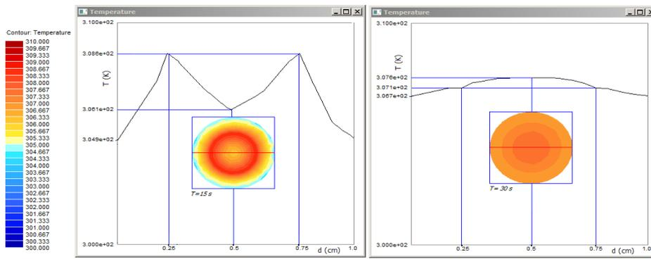
Fig. 7: Images of temperature for  $t=15$  s and  $t=30$  s across the specimen,  $d$  (normalized diameter).
