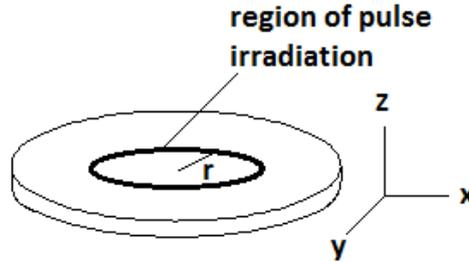
Fig. 1: Schematic diagram used in this work for measuring thermal diffusivity.
