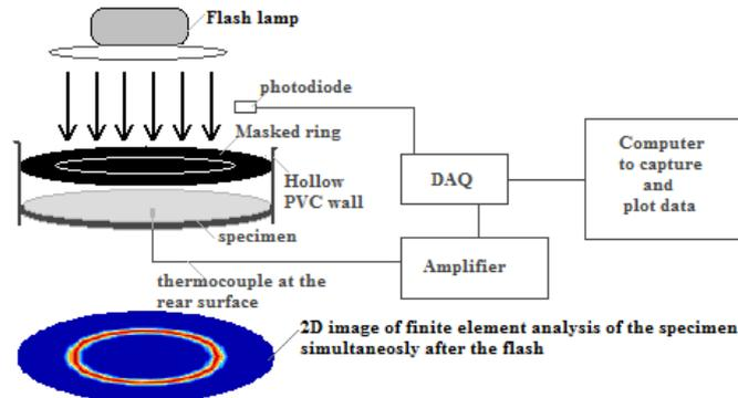
Fig. 3: Experiment setup for the present work to measure the thermal diffusivity of the foils.
