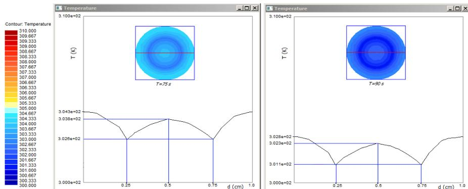
Fig. 9: Images of temperature for  $t=75$  s and  $t=90$  s across the specimen,  $d$  (normalized diameter).
