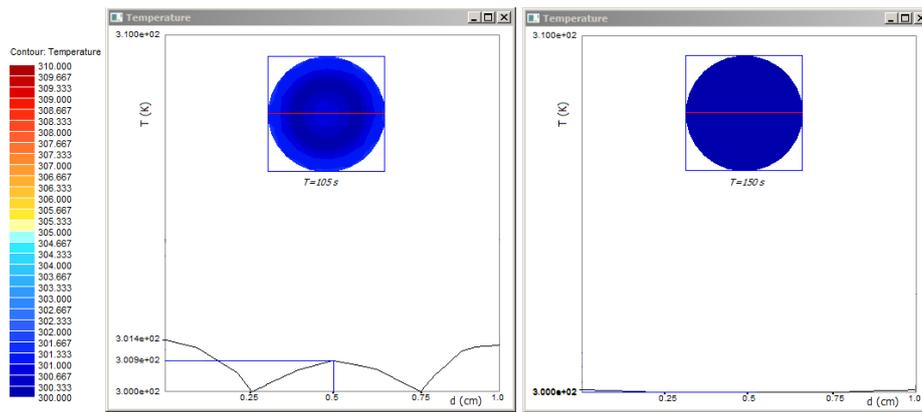
Fig. 10: Images of temperature for  $t=105$  s and  $t=150$  s across the specimen,  $d$  (normalized diameter).
