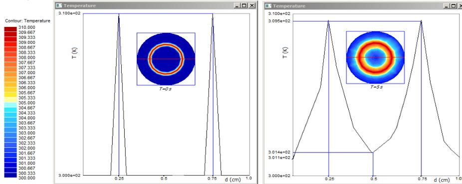
Fig. 6: Images of temperature for  $t=0$  s and  $t=5$  s across the specimen,  $d$  (normalized diameter).
