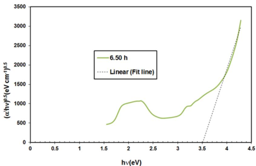
Fig. 4. Tauc's plot corresponding to indirect band gap for irradiated PANI samples at alpha particle irradiation time 6.50 h.
