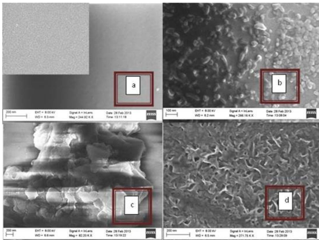
Fig. 1. Top-View FE-SEM images of synthesized PANI samples on glass substrate for virgin and irradiated by alpha particle with different irradiation times: (a) Virgin, (b) 6.50 h, (c) 41.00 h and (d) 71.00 h.
