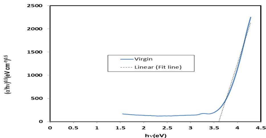
Fig. 3. Tauc's plot corresponding to indirect band gap for virgin PANI sample.
