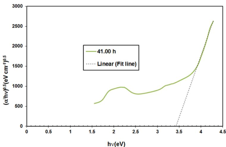
Fig. 5. Tauc's plot corresponding to indirect band gap for irradiated PANI samples at alpha particle irradiation time 41.00 h.
