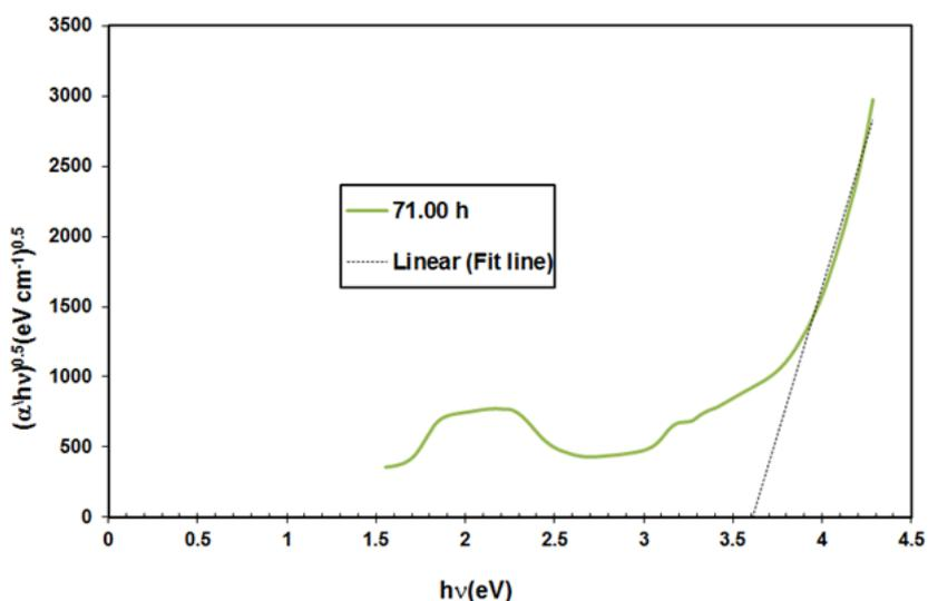
Fig. 6. Tauc's plot corresponding to indirect band gap for irradiated PANI samples at alpha particle irradiation time 71.00 h.
