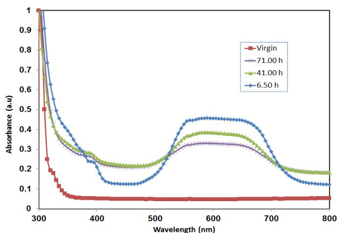
Fig. 2. UV- Vis spectra of the virgin and irradiated of nano-PANI samples with alpha particles at different irradiation times.
