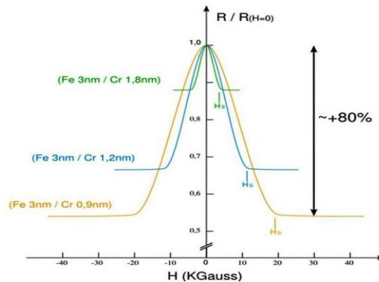
**Fig.3** the results from Fert’s original the current and the applied magnetic field are same axis in the plane of the layers.
