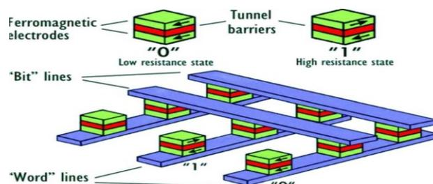
or the aligned state. MTJs took over from GMR devices in MRAM applications due to their high magneto resistance, high resistance, which makes them compatible with CMOS technology, ease of scaling to small dimensions and a weak variation with temperature. Developments in spin-transfer switching and the enhanced MR values found with crystalline and textured barriers have recently given new impetus to these developments.
