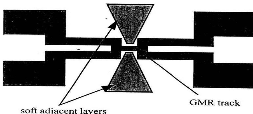
**Fig.5** Details of GMR device element
