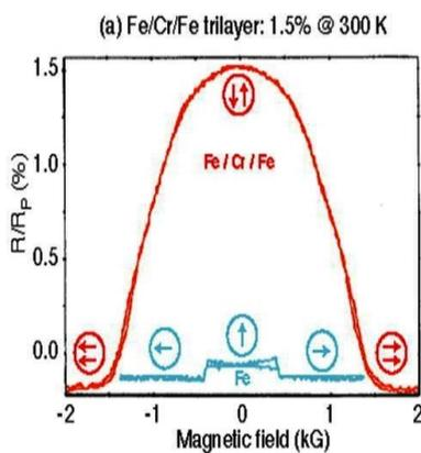
**Fig.2:** The results from Grunberg’s original paper. T = Paper. T= 4.2K room temperature. The current and the applied magnetic fields are along the same axis in the plane of the layers. [8] [1]
