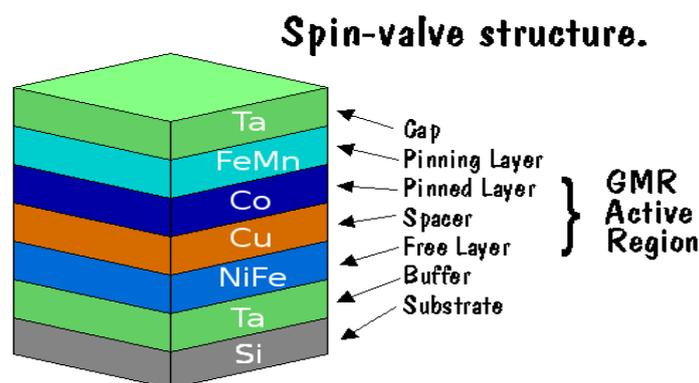
Fig.7. Spin Valves Sensors
