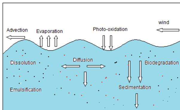
Figure 1: Oil spill processes
