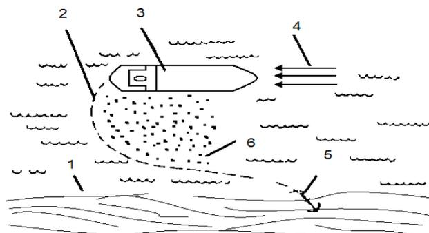
Figure 3.0: Mechanical method of containing oil spillage from an oil Tanker close to the bank of the river.
