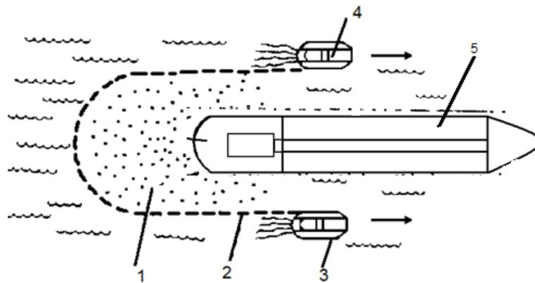
**Figure 3.2:** Mechanical method of containing and eventual cleaning of oil spillage in open waters.
