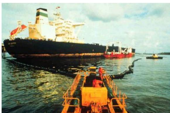
Figure 2.0: Oil booms used to contain oil spill from an oil tanker.
