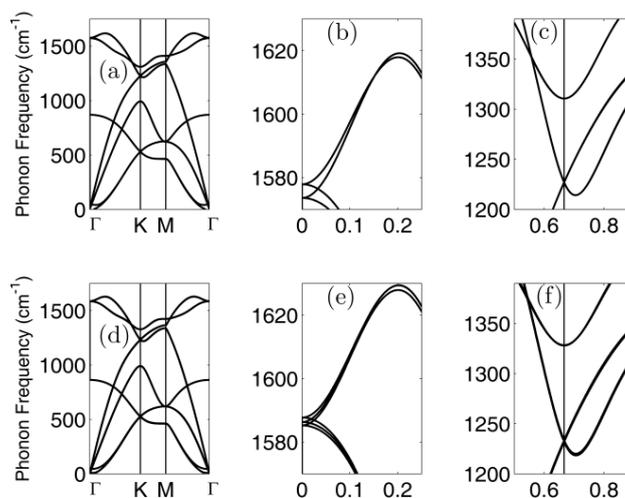
Figure. 7 below is the phonon dispersion of some FLGs calculated using C.blyp\_van.ak.UPF. Though the phonon frequencies in (a) and (d) appear degenerate except at the frequencies below  $200 \text{ cm}^{-1}$  however, (b), (e) and (f) show that all the frequencies are actually non-degenerate.
