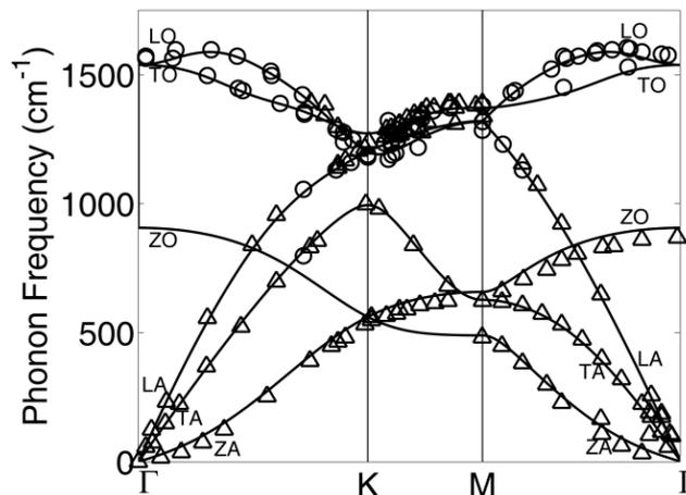
Figure 6: The phonon dispersion of graphene calculated using the pseudopotential C.pz-rrkjus.UPF. Circles are the INS data of Ref. [9], triangles are the IXS data of Ref. [10], and the solid line is our calculated points.
