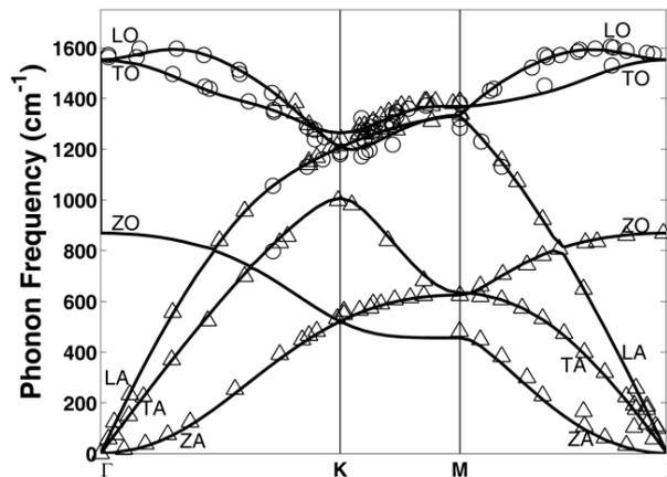
Figure 5: The phonon dispersion of graphene calculated using the pseudopotential C.pz-rrkjus.UPF. Circles are the INS data of Ref. [9] triangles are the IXS data of Ref. [10] and the solid line is our calculated points.
