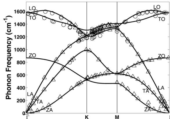
Figure 4: The phonon dispersion of graphene calculated using the pseudopotential C\_pbe-van\_bm\_UPF. Circles are the INS data of Ref. [9] triangles are the IXS data of Ref. [10].
