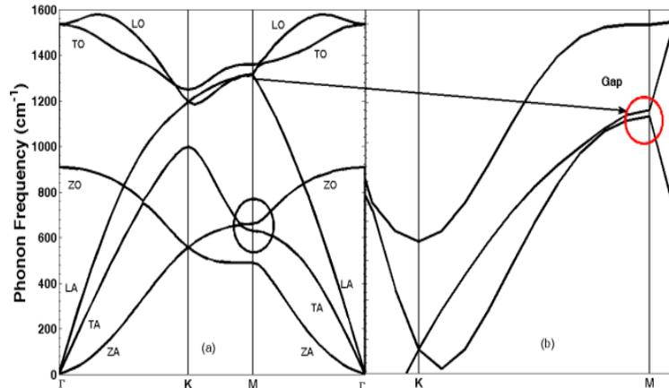
Figure 2: Phonon Dispersion of Graphene. (a) The phonon dispersion in the KM-direction and (b) Magnified view of the Optical Phonon in the KM direction. Observe the circled gaps in the two figures: in (a), ZO and TA cross each other before the special symmetry point M while the gap shown in the magnified view in (b) is not conspicuous in (a).
