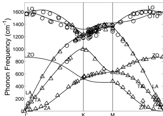
Figure 3: Calculated Phonon dispersion of graphene fitted to the IXS data of Ref. [10] (triangles) and the INS data of Ref. [9] (circles).
