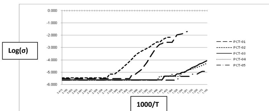
Fig No. 9 : d.c conductivity curve for Calcium modified Lead Titanate
