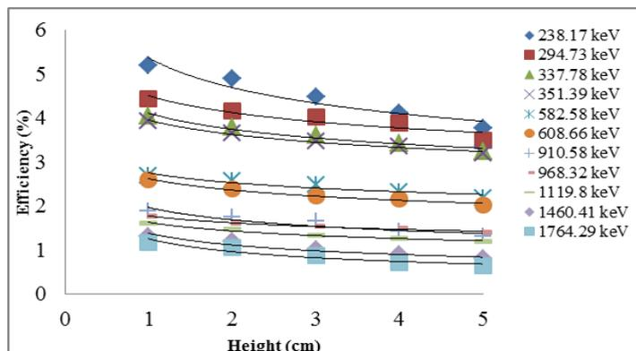
Fig. 05: Height vs. Efficiency curve for sample STDMC
