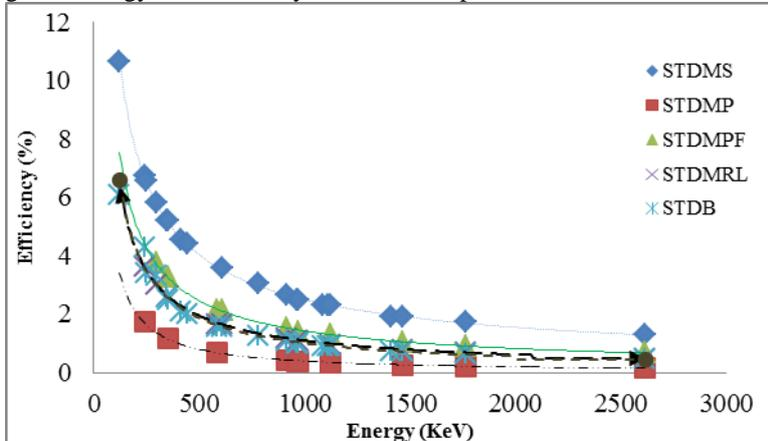
Fig. 04: Energy vs. Efficiency curve for samples at 5cm distance from the Detector 2 surface.
