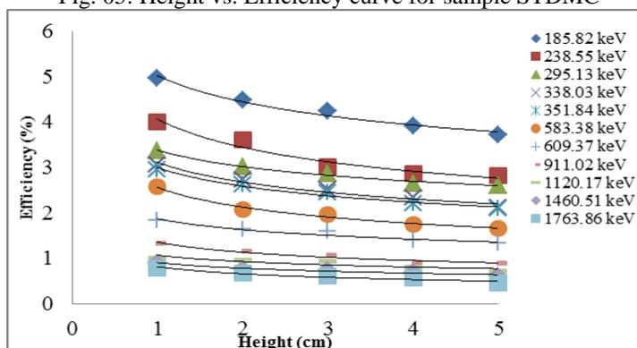
Fig. 06: Height vs. Efficiency curve for sample STDMG
