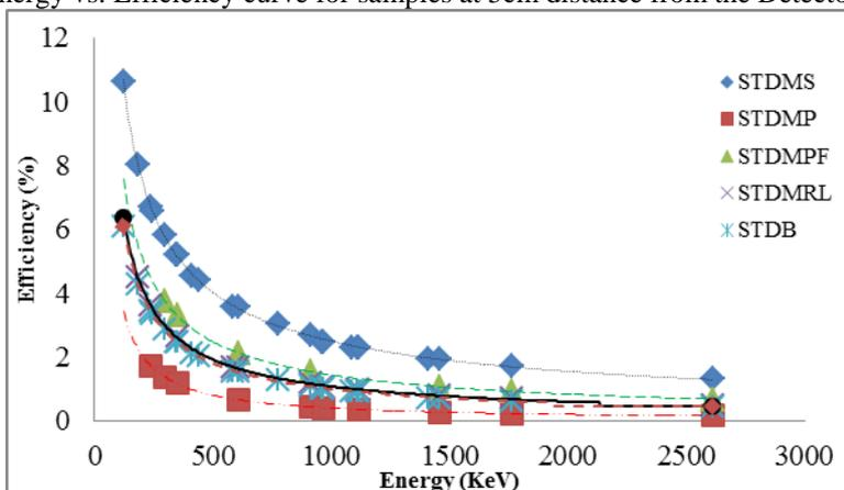
Fig. 03: Energy vs. Efficiency curve for samples at the surface of detector 2.
