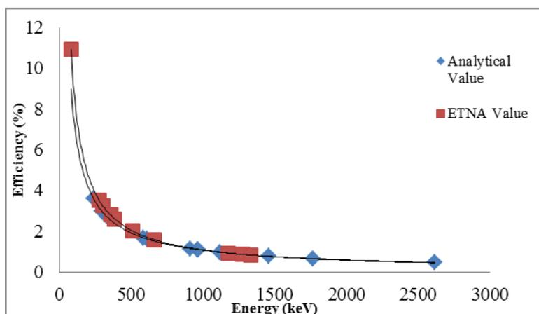
Fig. 10: Comparison between analytical and ETNA efficiency value for sample STDML.
