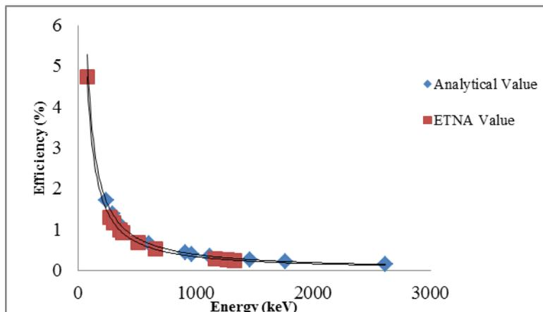
Fig. 08: Comparison between analytical and ETNA efficiency value for sample STDMP.
