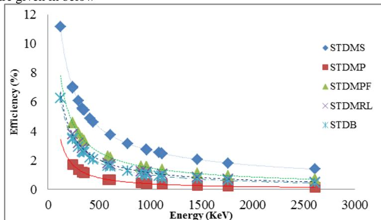
Fig. 01: Energy vs. Efficiency curve for samples at the surface of detector 1.
