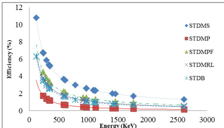
Fig. 02: Energy vs. Efficiency curve for samples at 5cm distance from the Detector 1 surface.
