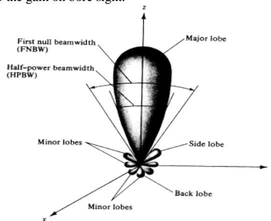
In order to find the absolute gain in any direction the gain on bore sight must be known. If this gain is expressed in decibels then this value can simply be added to the gain at any point to gain the absolute gain. The absolute gain on bore sight is measured by comparison with a standard gain antenna, which functions as a reference antenna whose gain is calculated or measured with a high degree of accuracy.
