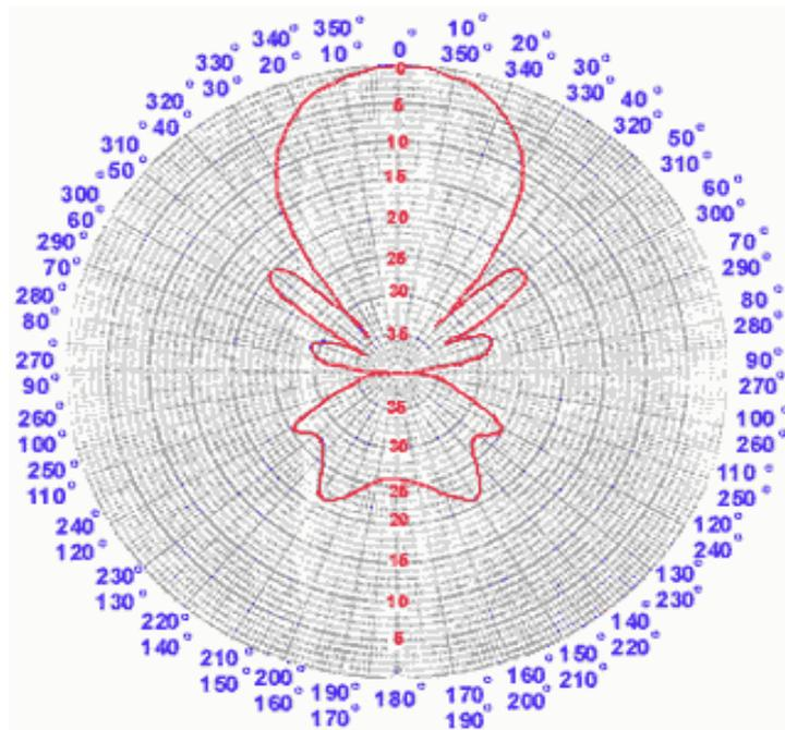
**1.2.3 Beam width-** The beam width (or half power beam width) of an antenna is typically defined for each of the principle plane as the angle between the point in the main lobes that are down from the maximum gain by 3dB.
