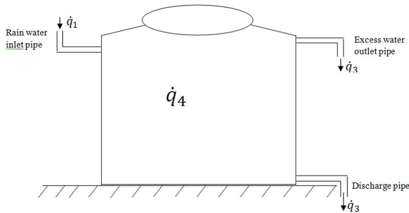
Fig 3.2: The tank model
