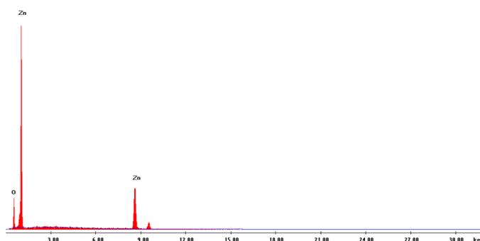
**Fig3: EDX of ZnO nano particles**
