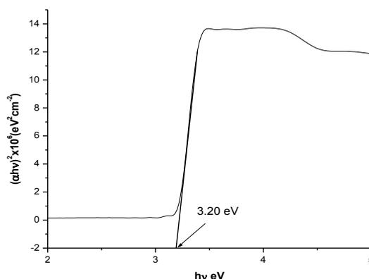
Fig 5:Tauc plot for determination of band gap
