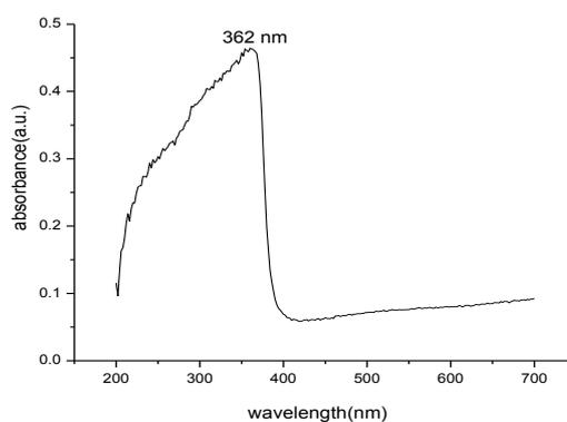
Fig4: DRS of synthesized ZnO nanoparticles
