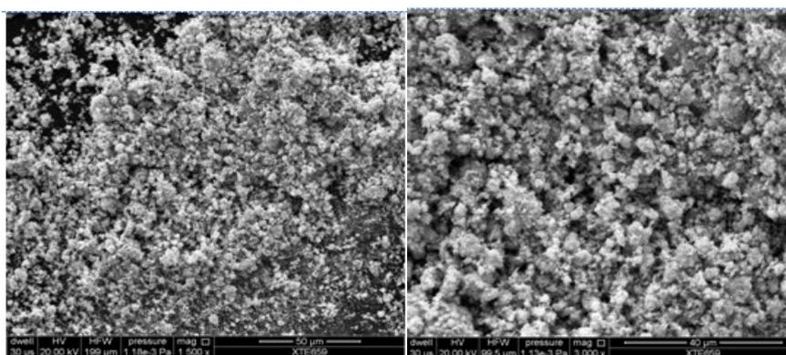
**Fig2: SEM image of ZnO nanoparticles**
