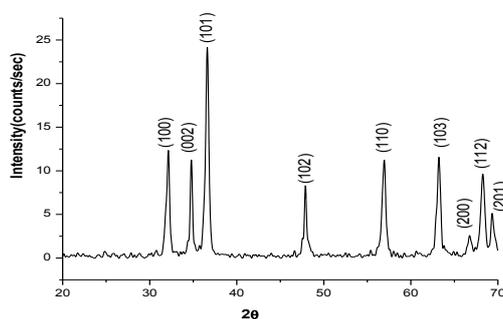
Fig1: XRD patterns of synthesized ZnO nanoparticles
