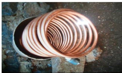
Figure 3: Heat exchanger during assembly
