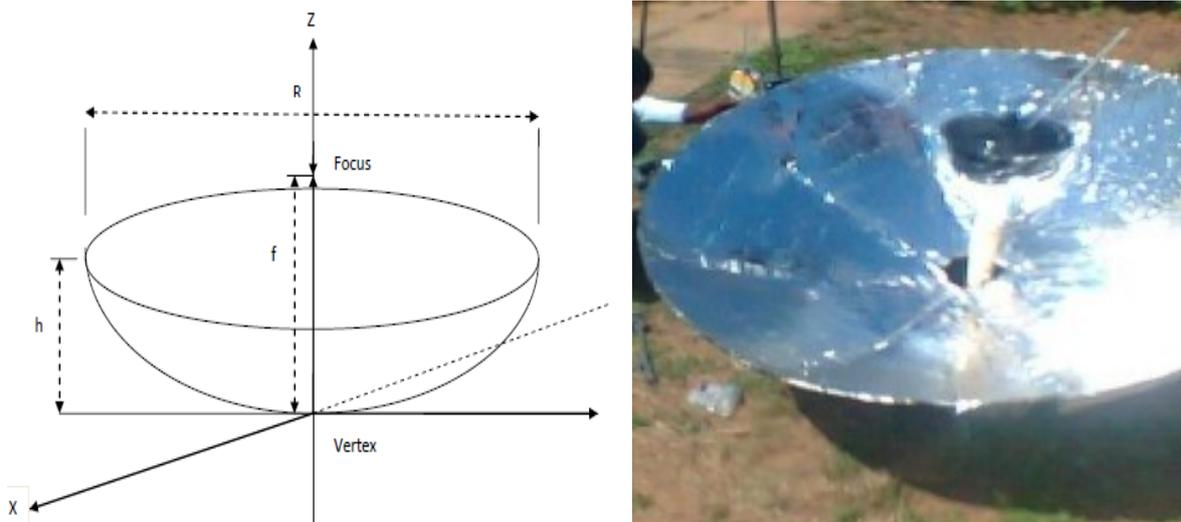
**Figure 1:** Schematic and the constructed views of the solar parabolic dish collector cooker
