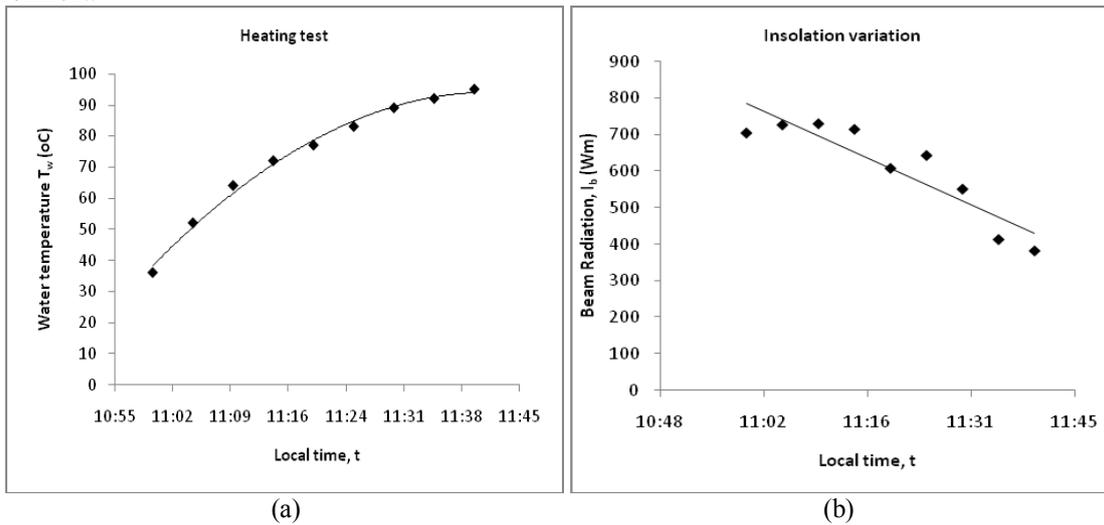
Figure 3: Graphs of water temperature (a) and global insolation (b) against local time
