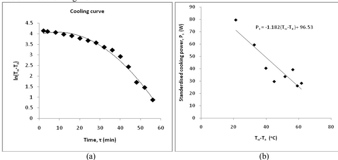
Figure 4: cooling curve (a) and a plot of standardised cooking power against difference in temperature (b)
