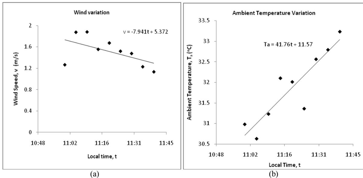
**Figure 2:** Wind speed (a) and ambient temperature (b) variation with local time on the day of experiment. The cooking power P of the parabolic solar cooker which is the rate of useful energy available during heating period is given as:
