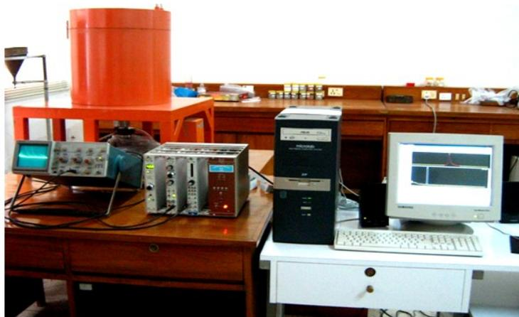
Fig. 4 High Purity Germanium (HPGe) detector system for sample analysis
