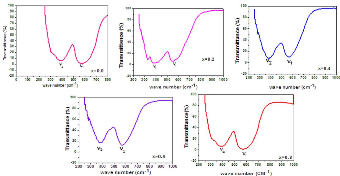
Figure (2) FTIR spectra of  $\text{Ni}_{0.2}\text{Cu}_x\text{Zn}_{0.8-x}\text{Fe}_2\text{O}_4$  ( $x=0.0$  to  $0.8$ ) ferrite nano-particles.
