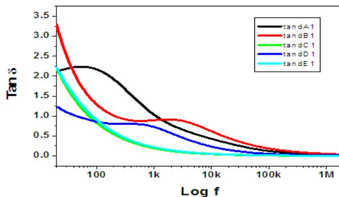
Figure (5): Variation of dielectric loss tangent with frequency
