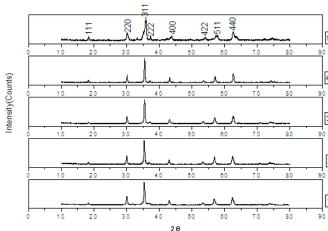
Fig 1 XRD pattern of Cu substituted Ni-Zn nanoferrites.
