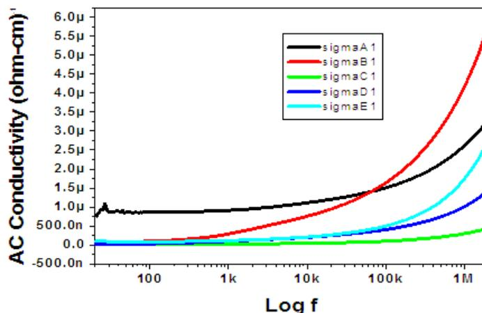
Figure (6): Variation of ac conductivity with frequency.
