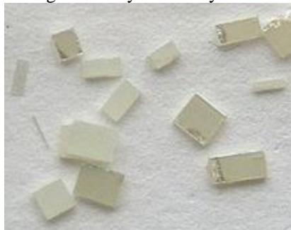
Synthetic single crystals of TiO<sub>2</sub>, ca. 2–3 mm in size, cut from a larger plate.
