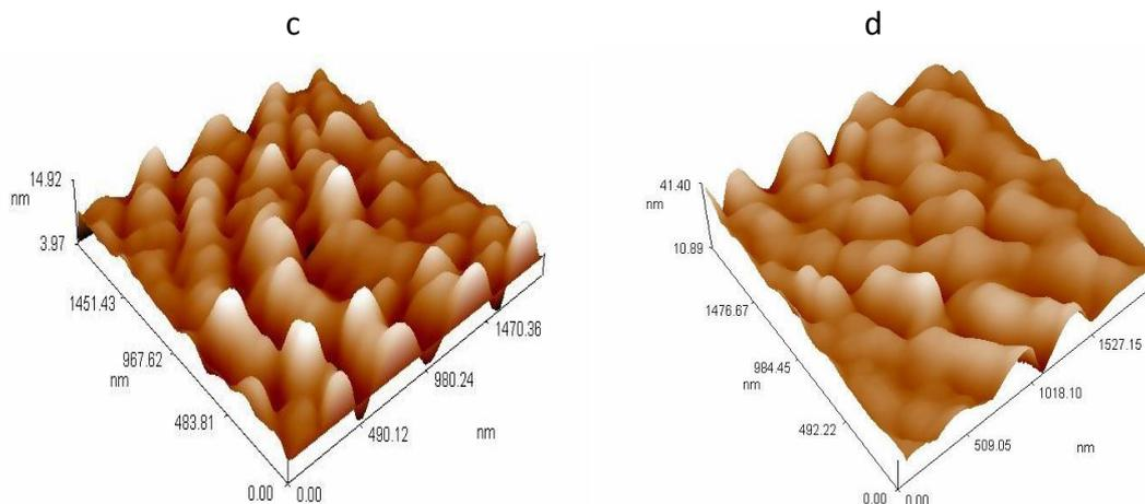
**Fig. 5:** AFM studies on deposited ZnO thin films at different substrate temperature a)473K, b)513K, c)573K and d)673K showing different structure.
