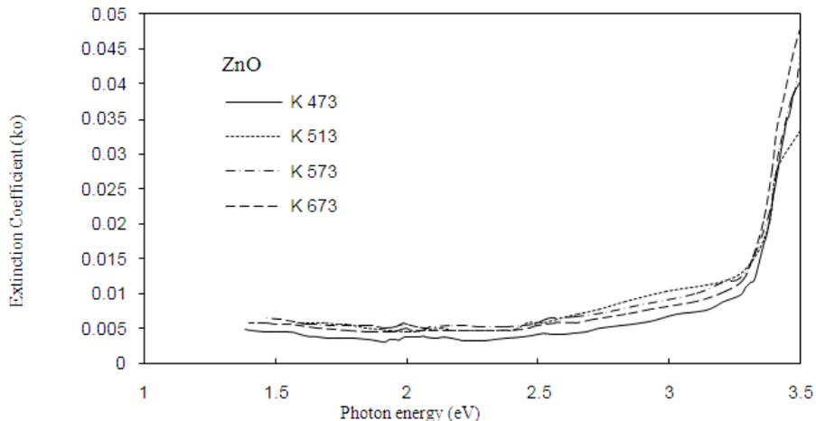
**Fig. 4:** Variation of extinction coefficient with photon energy.
