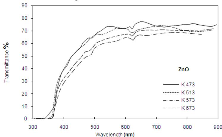
**Fig. 1:** Optical transmittance spectra of ZnO thin film on fused quartz glass.
