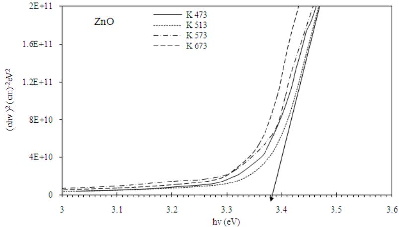
**Fig. 2:** Plot of  $(ahv)^2$  vs. photon energy  $(hv)$  for ZnO films grown at various substrate temperatures
