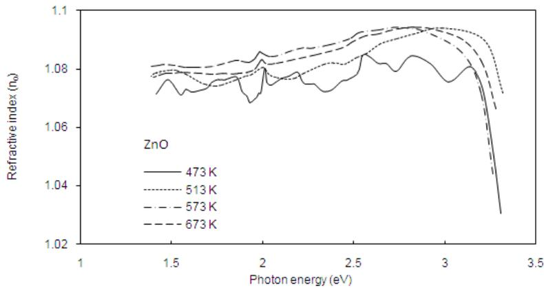
**Fig. 3:** Variation of refractive index with photon energy.
