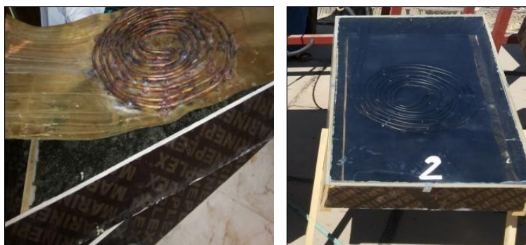
Figure (7) A design solar collector shaped – 2 copper tubes parallel a circular path connected and starts from the center
