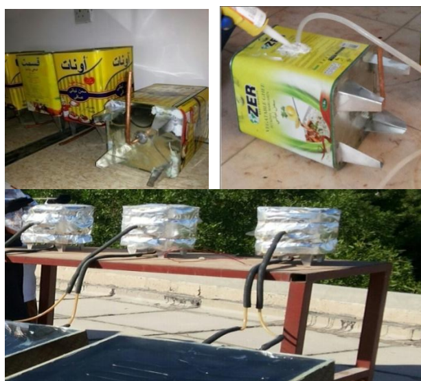
Figure (1) Fabrication method a tank which to connected with the solar collector .
