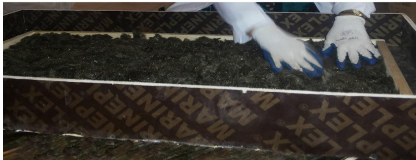
Figure (4) Show the how to put the glass wool under the copper plate.
