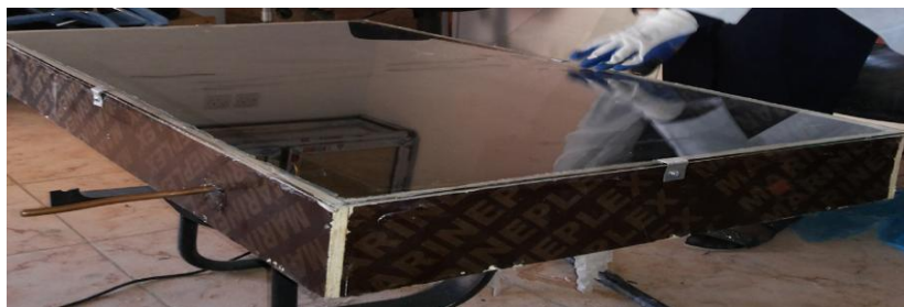
Figure (5) Show the installation of the glass cover on the wooden box .
