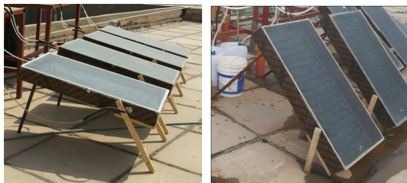
( 15^{\circ} ) in summer ( 45^{\circ} ) in winter Figure (2) Solar collector angle in the summer and winter facing the sun .
