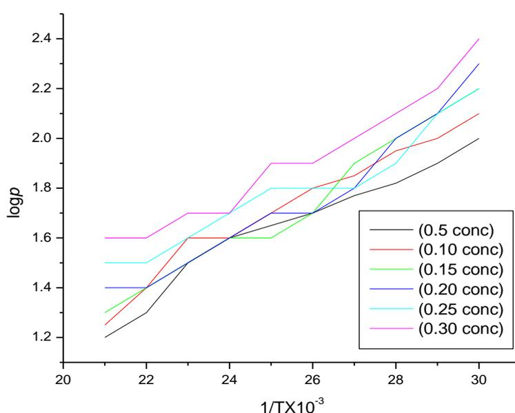
**Fig.2 : log ρ Vs 1/T at various La<sup>3+</sup> substituted concentrations**
