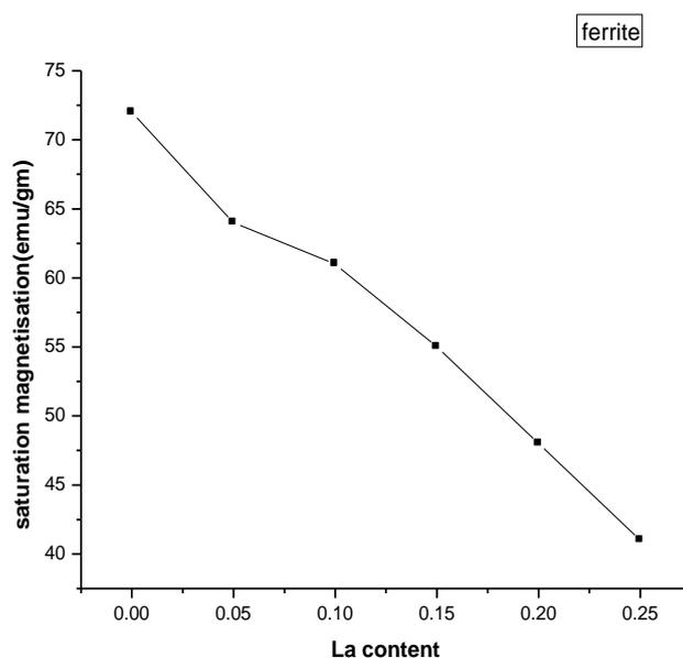
**Fig.6: Variation of Saturation Magnetization with La content**
