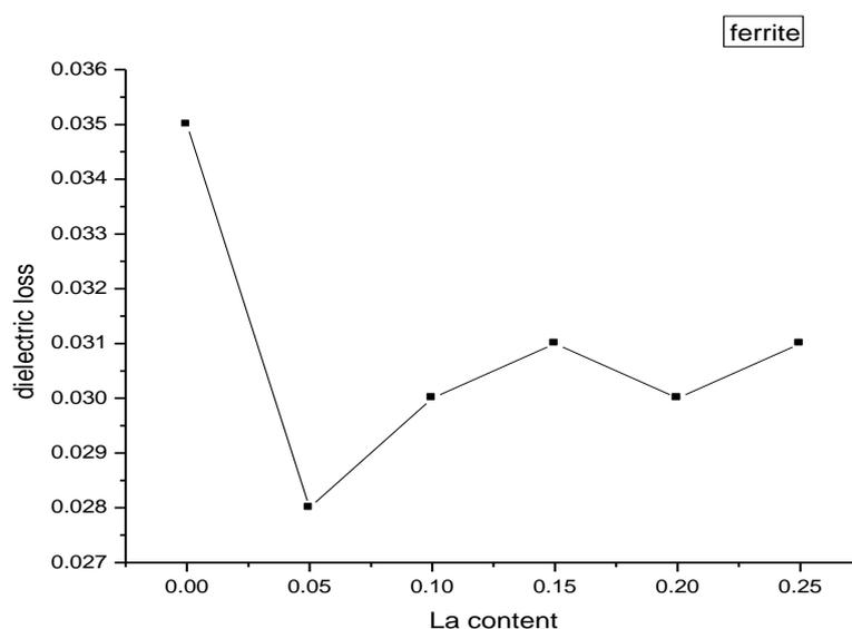
**Fig.5:** variation of dielectric loss with la content
