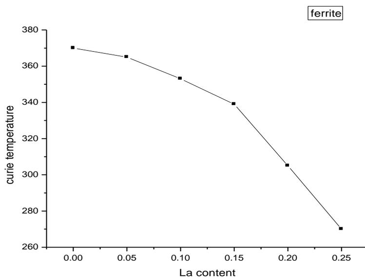
**Fig 3: Variation of Curie temperature with La content**
