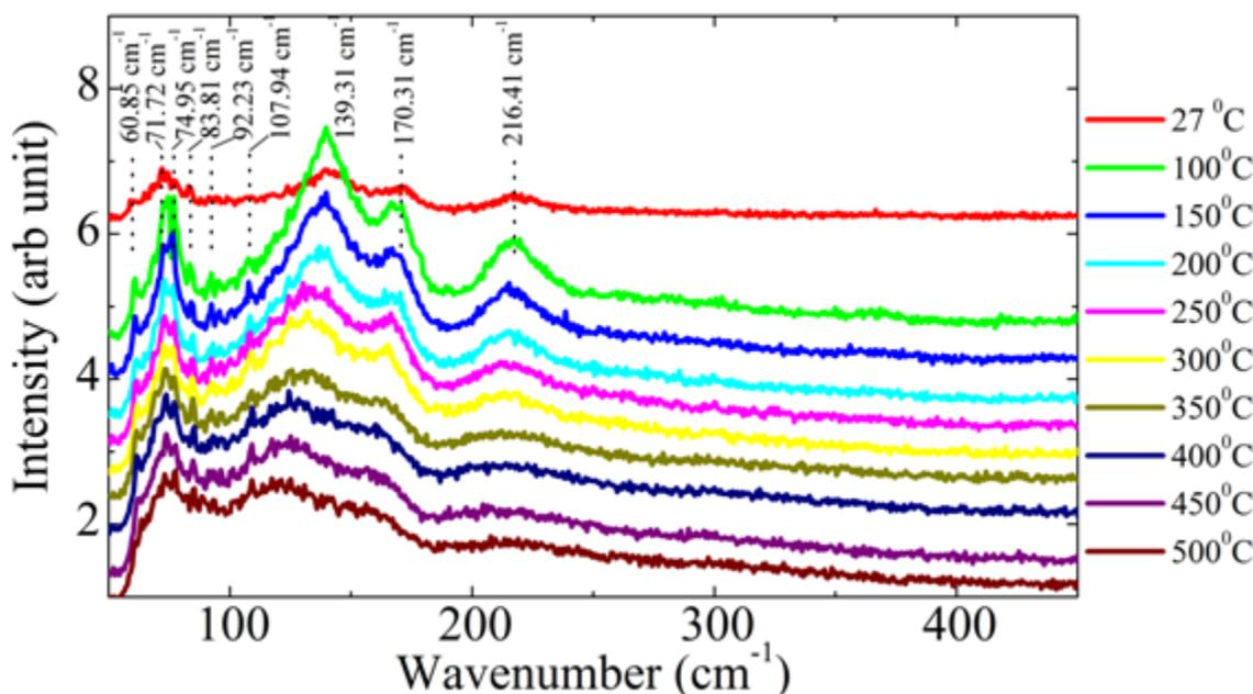
**Figure 1.** A typical Raman spectrum of BFO sample indicating various Raman active modes.
