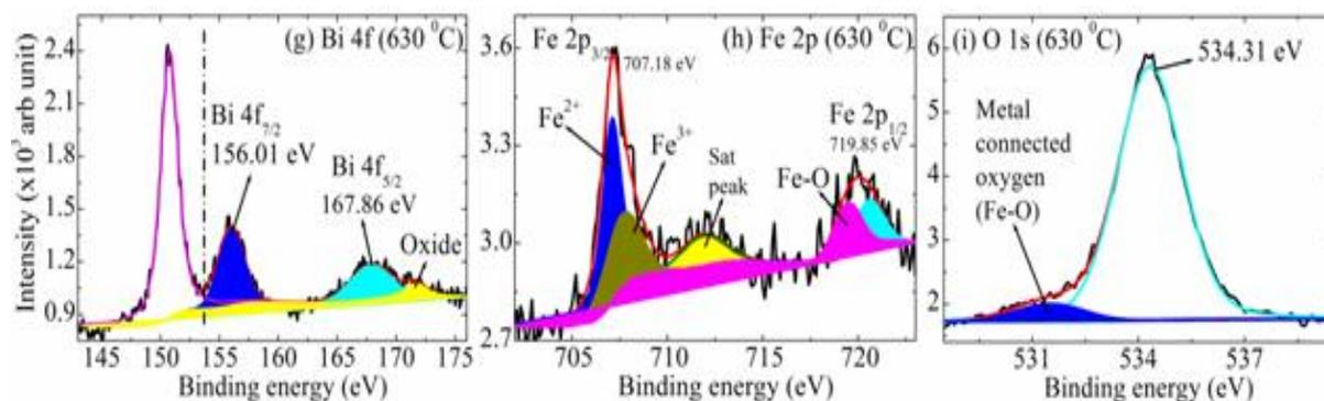
**Figure 3.** Typical XPS spectra of BFO thin film where as it is spectra are (a) Bi 4f, (b) Fe 2p, (c) O 1s; spectra annealed at 430 °C (d) Bi 4f, (e) Fe 2p, (f) O 1s and the spectra annealed at 630 °C are (g) Bi 4f, (h) Fe 2p, (i) O 1s.
