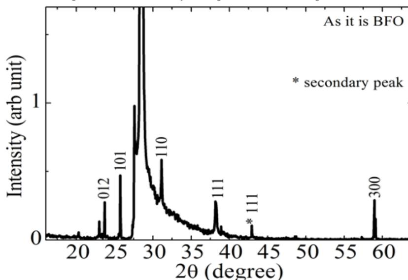
**Figure 4.** X-ray diffraction pattern of BiFeO<sub>3</sub> compound deposited on Si (111) substrate.
