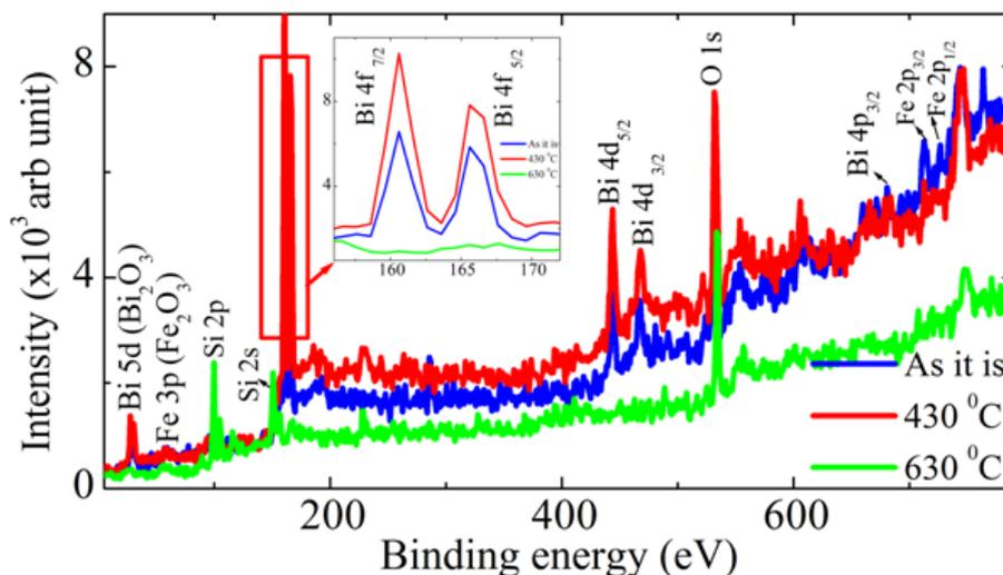
**Figure 2.** Typical full scale XPS spectra of BFO thin film
