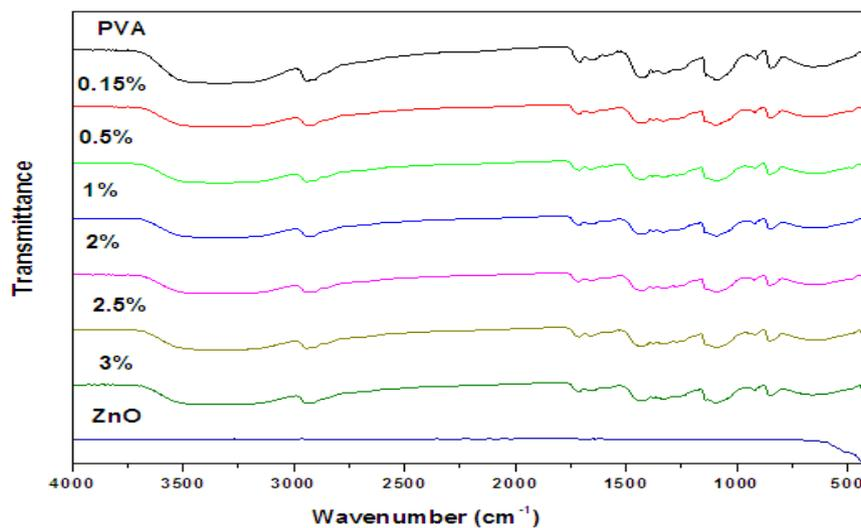
Fig. (2): FTIR spectra of: PVA, ZnO/ PVA films, and ZnO respectively.
