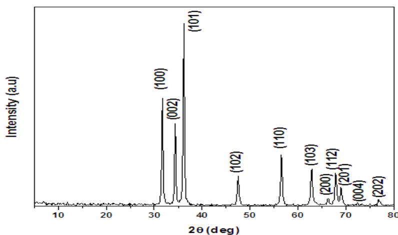
Fig. (1b): XRD pattern of pure ZnO.
