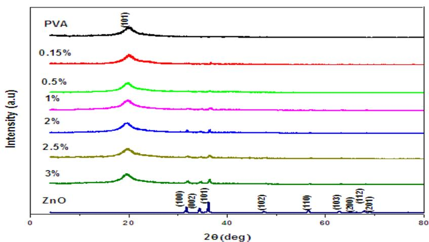
Fig. (1c): XRD pattern of PVA ZnO/ PVA films, and ZnO respectively.
