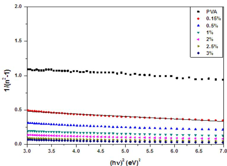
Fig. (6): Relation between  $1/(n^2 - 1)$  and  $(hv)^2$  for pure PVA and ZnO/ PVA nanocomposites.
