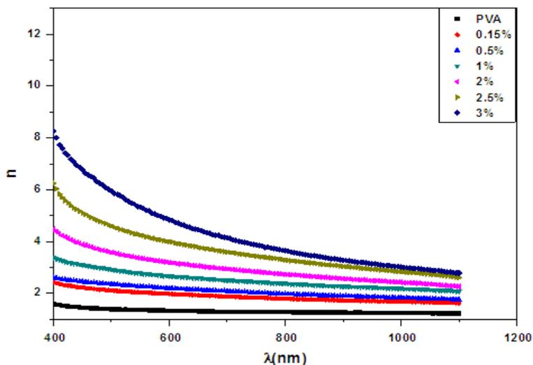
Fig. (5): The refractive index of pure PVA and ZnO/ PVA nanocomposite films.
