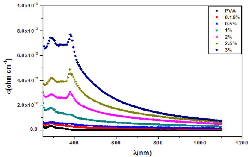
Fig. (9): The optical conductivity of pure PVA and ZnO/ PVA nanocomposite films.
