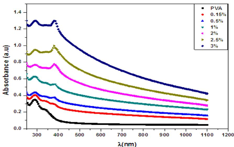
Fig. (3): UV-visible absorption spectra of pure PVA and ZnO/ PVA nanocomposite films.
