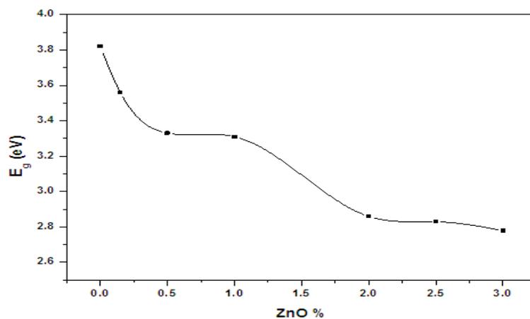
Fig. (4b): The obtained values for optical band gap as a function of ZnO concentration.
