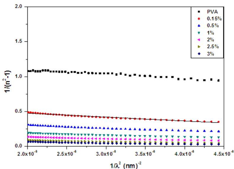
Fig. (7): Relation between  $1/(n^2 - 1)$  and  $(1/\lambda^2)$  for pure PVA and ZnO/ PVA nanocomposite films.
