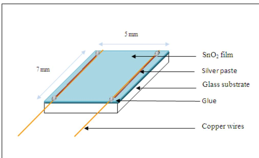
**Figure 1:** Schematic diagram of sensor element
