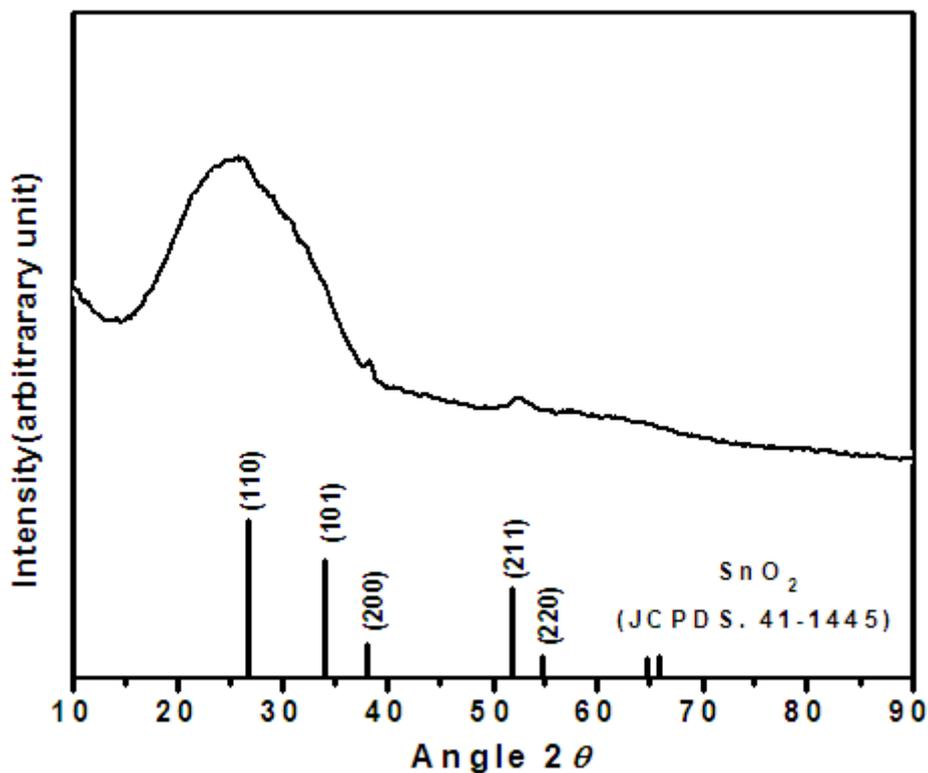
Figure 4: X-ray powder pattern of spray deposited SnO<sub>2</sub> film on glass slide.
