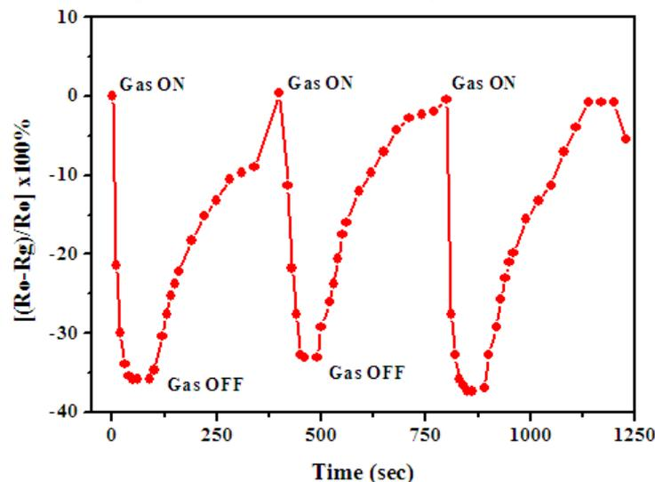
Figure 8: Gas response of SnO<sub>2</sub> film loaded in prepared setup @ 110°C recorded for H<sub>2</sub>S
