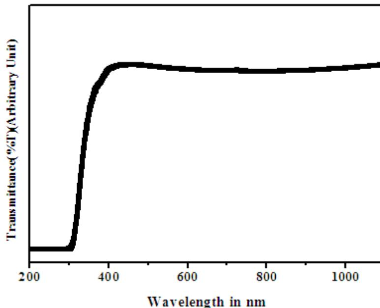
Figure 6: Optical transmittance spectrum of  $\text{SnO}_2$  thin film of glass slide.
