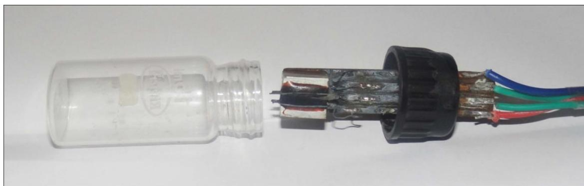
**Figure 3:** Photograph of gas sensor setup
