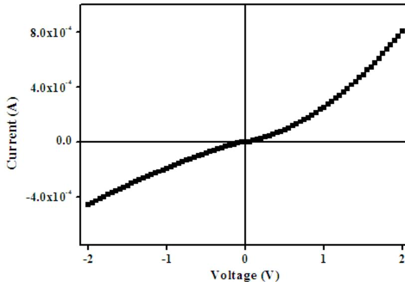
Figure 7: Current – Voltage (I–V) curve of SnO<sub>2</sub> thin film.
