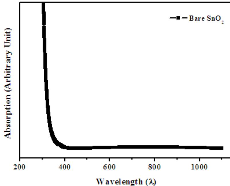
Figure 5: Optical absorption of  $\text{SnO}_2$  thin film recorded between 300 nm to 1100 nm.
